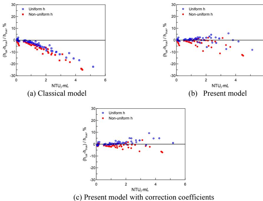
**Figure 6:** Comparison of errors in the prediction of the pure-heat transfer coefficient according to the models and the uniform and non-uniform heat transfer coefficients. (a) Classical model, (b) Present model using coefficients  $c_1=1$  and  $c_2=0$  in the modified fin efficiency  $\eta_x$ , (c) Present model using coefficients  $c_1=1.05$  and  $c_2=0.008$  in the modified fin efficiency  $\eta_x$
