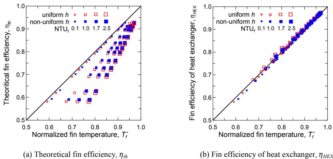
**Figure 4:** Comparison of the fin efficiencies and the normalized fin temperature for the uniform and non-uniform heat transfer coefficients.
