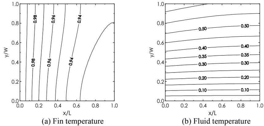
**Figure 3:** Fin and fluid temperature distribution in the reference condition on Table 1,  $mL = 0.5$ ,  $NTU_f = 1$ , uniform heat transfer coefficient ( $\eta_{th} = 0.924$ ,  $\varepsilon/\varepsilon_{fa} = 0.948$ ,  $T_f^* = 0.952$ ).
