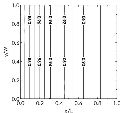
**Figure 2:** Fin temperature distribution of external flow condition,  $mL=0.5$ ,  $NTU_f=0.1$ , ( $\eta_{th} = T_f^* = 0.924$ ).
