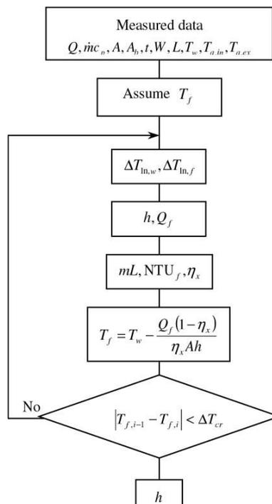
Figure 7: Procedure to obtain the pure heat transfer coefficient for the heat exchanger.
