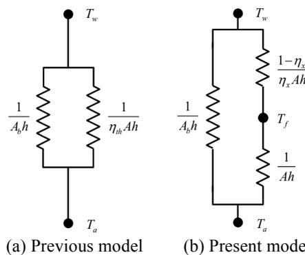
**Figure 5:** Thermal resistance models for the heat exchanger.
