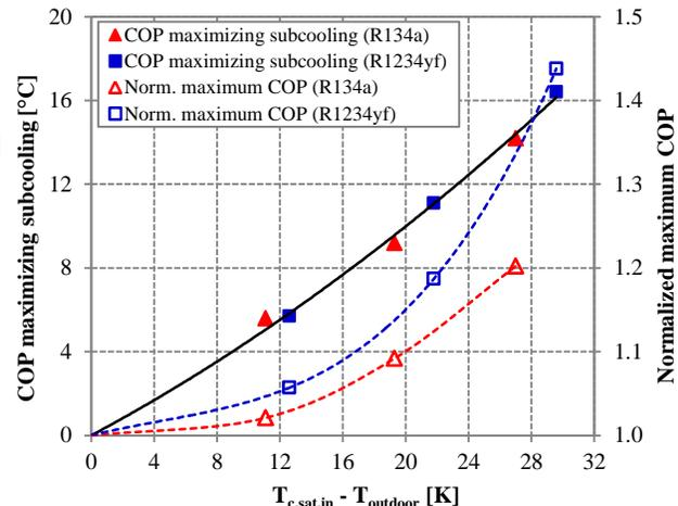
**Figure 9:** COP maximizing subcooling and normalized maximum COP (with respect to COP at zero subcooling) as a function of the temperature difference between outdoor and condensing refrigerant at maximized COP conditions, for R134a and R1234yf.
