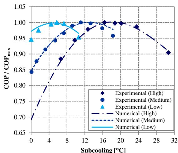
**Figure 13:** Experimental validation of the normalized COP predicted by the model (R1234yf)
