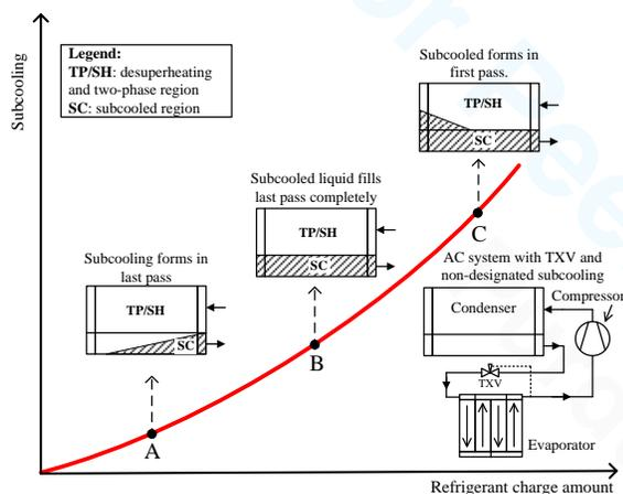
**Figure 2:** Typical variation of the subcooling with the refrigerant charge in a non-designated area
