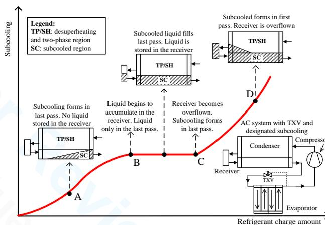
**Figure 3:** Typical variation of the subcooling with the refrigerant charge in a designated area
