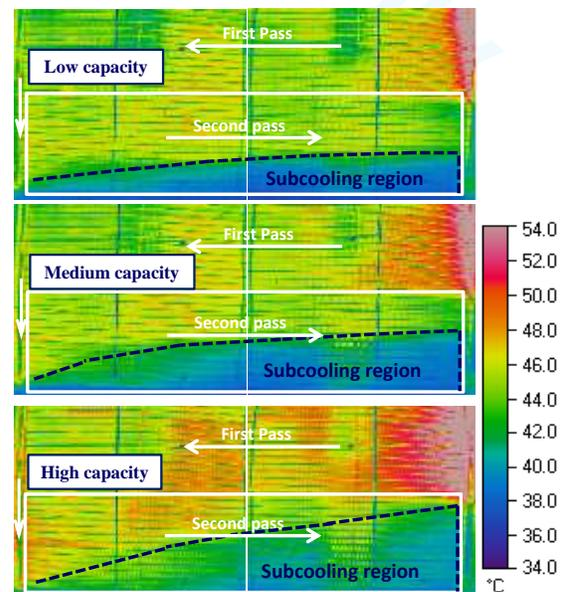
**Figure 7:** Infrared images taken at the inlet surface of the condenser at COP maximizing subcooling for high, medium and low cooling capacities. Dashed lines indicate approximately the area occupied by the subcooled liquid.
