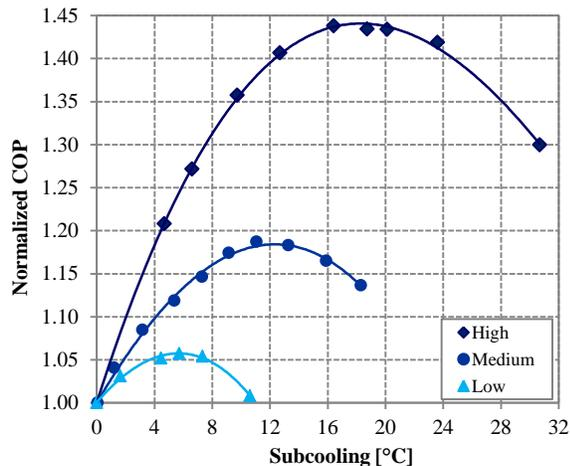
**Figure 8:** Normalized COP as a function of the condenser subcooling for high, medium and low cooling capacities (R1234yf)
