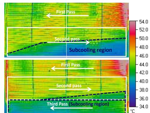
**Figure 12:** Infrared images from the inlet surface of NDA (top) and DA (bottom) condensers at a subcooling of 10°C for the medium cooling load. Dashed lines to indicate approximately the area occupied by the subcooled liquid.
