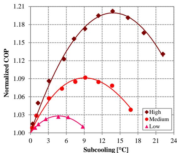
**Figure 5:** Normalized COP as a function of the condenser subcooling for high, medium and low cooling capacities (R134a)
