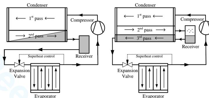
**Figure 4:** System setups for subcooling obtained in a non-designated (left) and a designated area (right) of the condenser
