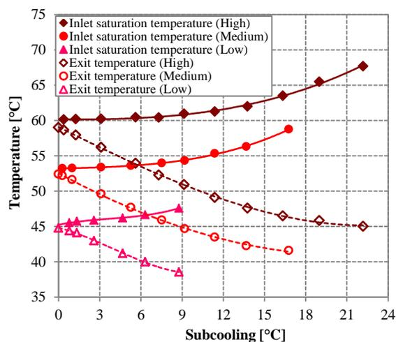
**Figure 6:** Inlet saturation temperature and exit temperature of the refrigerant as a function of the condenser subcooling for high, medium and low cooling capacities (R134a)
