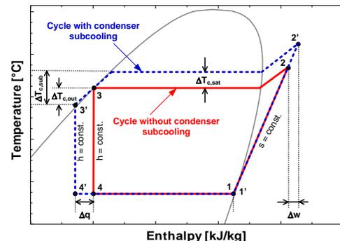
Figure 1: Comparison between theoretical cycles with and without condenser subcooling
