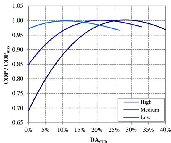
Figure 14: Numerical results for normalized COP as a function subcooling area ratio (R1234yf)
