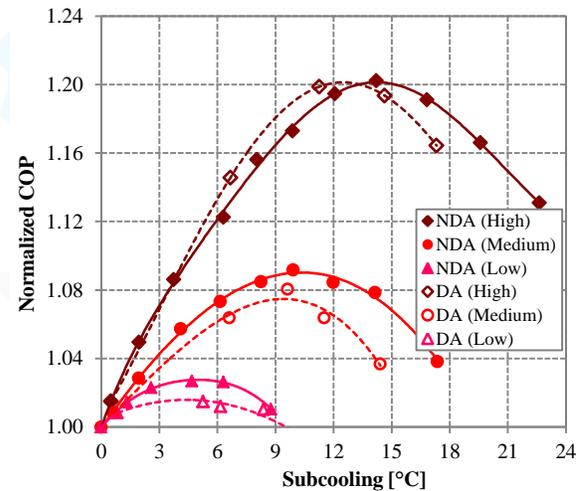
**Figure 11:** Normalized COP as a function of the condenser subcooling for designated (DA) and non-designated subcooling (NDA), at high, medium and low cooling loads (R134a).
