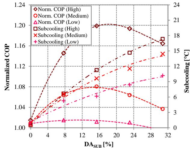
**Figure 10:** Normalized COP and condenser subcooling as a function of the ratio between the subcooling designated area ratio for high, medium and low cooling loads (R134a).
