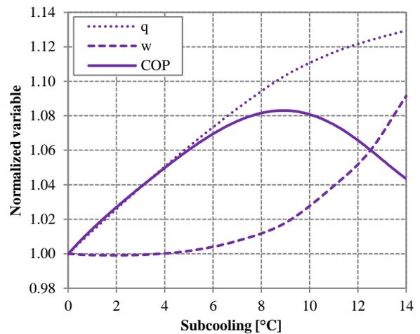
**Figure 6:** Effect of condenser subcooling on normalized COP, refrigerating effect and specific compression work at outdoor and indoor temperatures of 35°C and 27°C (R1234yf)
