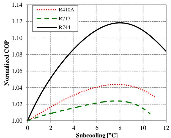
**Figure 8:** Effect of condenser subcooling on normalized COP for R744, R410A and R717, at outdoor and indoor temperatures of 35°C and 27°C
