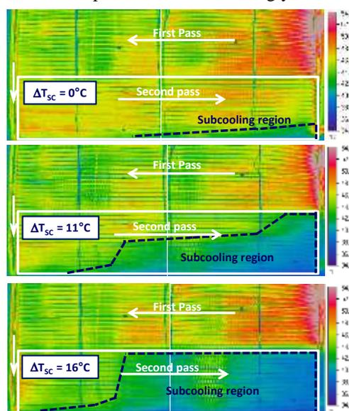
**Figure 10:** Infrared images at the inlet surface of the condenser for various degrees of subcooling with dashed lines to approximately indicate the area occupied the subcooled liquid (experimental).
