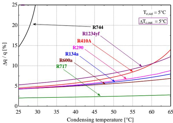
**Figure 3:** Effect of the condensing temperature on the relative gain in refrigerating effect for a  $\Delta T_{c,out} = 5^\circ\text{C}$ .
