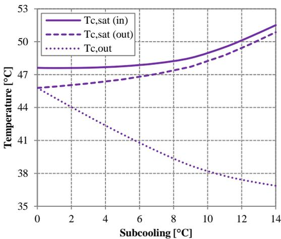
**Figure 5:** Effect of condenser subcooling on refrigerant temperatures at the condenser at outdoor and indoor temperatures of 35°C and 27°C (R1234yf)
