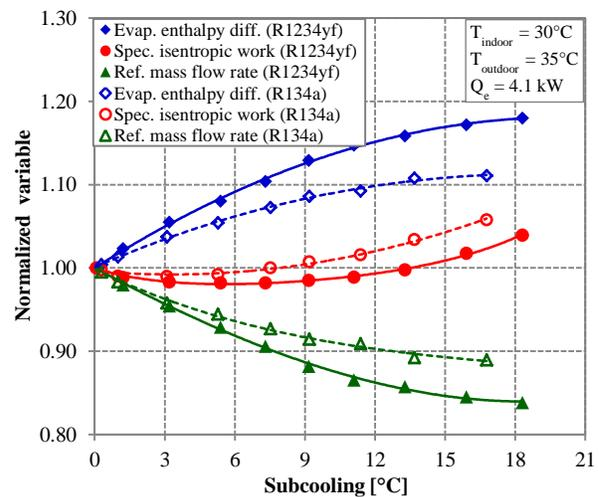
**Figure 12:** Effect of condenser subcooling on normalized refrigerant enthalpy difference across the evaporator, specific isentropic compression work and refrigerant mass flow rate, for R134a and R1234yf (experimental).
