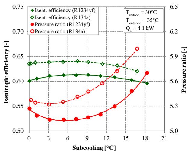
**Figure 13:** Effect of condenser subcooling on isentropic efficiency and compressor pressure ratio for R134a and R1234yf (experimental).
