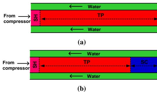
Figure 1: Schematic of a water-cooled condenser with (a) and without (b) subcooling.
