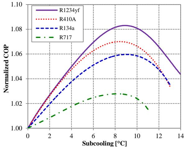
**Figure 7:** Effect of condenser subcooling on normalized COP for R717, R134a, R410A and R1234yf, at outdoor and indoor temperatures of 35°C and 27°C
