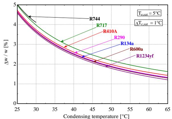
**Figure 4:** Effect of the condensing temperature on the relative increase in isentropic compression work for a  $\Delta T_{c,sat} = 1^\circ\text{C}$ .
