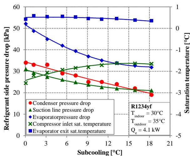
**Figure 14:** Effect of condenser subcooling on refrigerant side pressure drops and saturation temperatures (at the evaporator exit and compressor inlet) for R1234yf (experimental).
