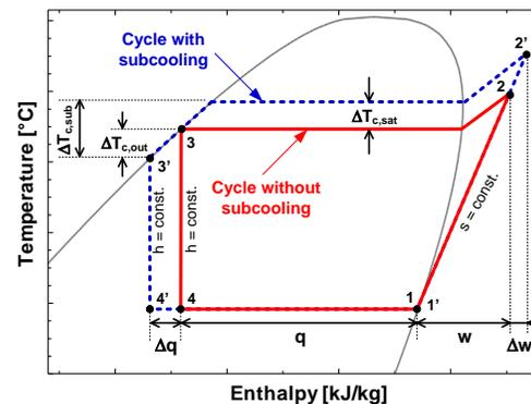
Figure 2: Schematic of cycles with and without subcooling in a T-h diagram.
