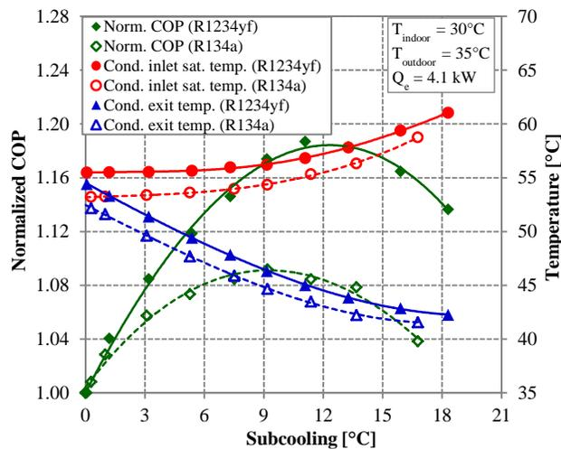
**Figure 11:** Effect of condenser subcooling on normalized COP, inlet saturation and exit temperatures of the refrigerant in the condenser for R134a and R1234yf (experimental).
