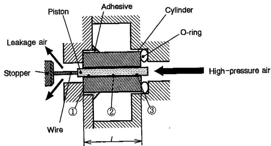
Figure 5 Test of leakage through the clearance between piston and cylinder
