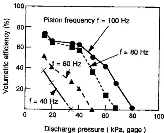
Figure 3 Experimental volumetric efficiency at various piston frequency (without oil)
