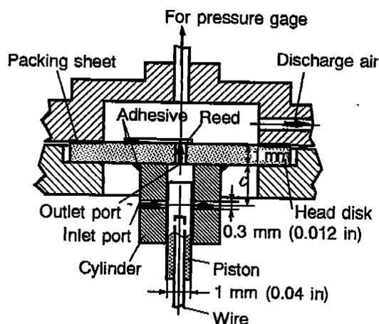
Figure 1 Schematic view of microcompressor
