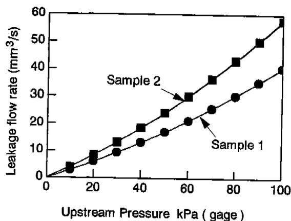
Figure 6 Results of leakage test
