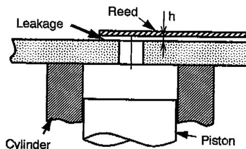
Figure 7 Reed valve clearance
