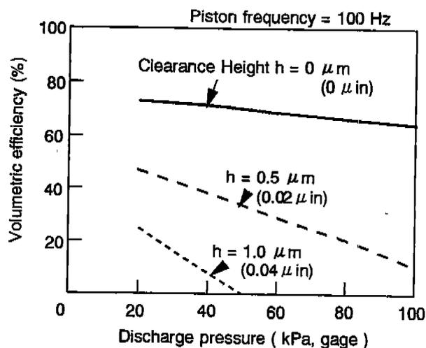
Figure 8 Effect of reed valve clearance on volumetric efficiency (simulation)
