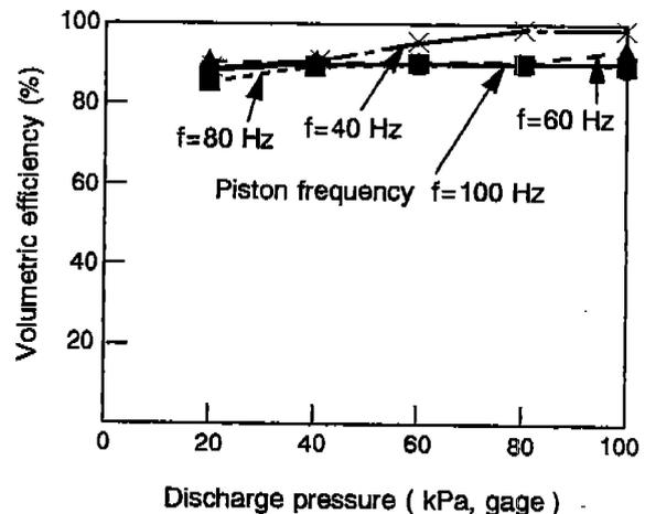
Figure 4 Experimental volumetric efficiency when oil is supplied
