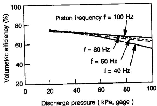
Figure 2 Calculated volumetric efficiency of the microcompressor from the simulation
