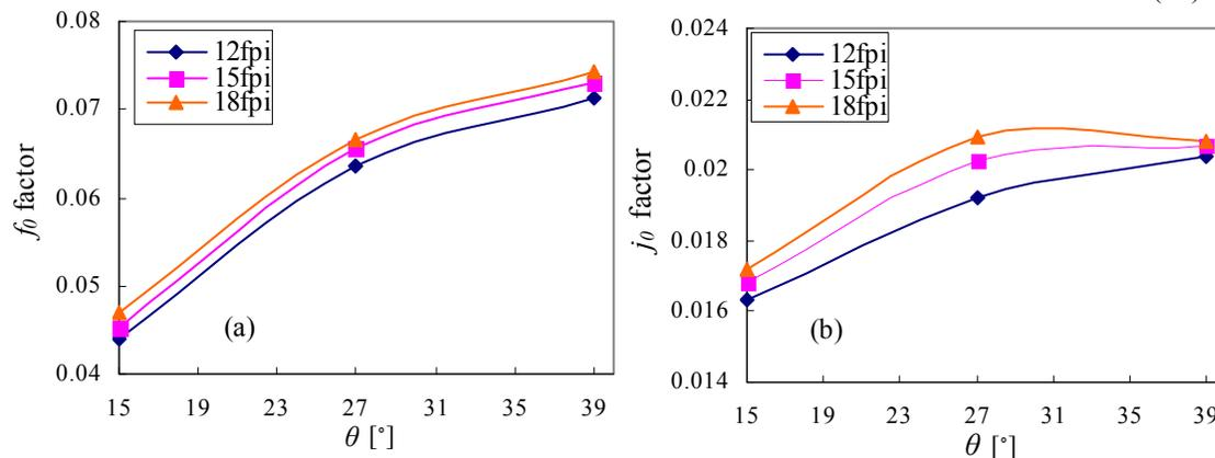
Fig. 6: Effect of louver angle  $j_0$  and  $f_0$  factors at the beginning of the first frosting cycle
