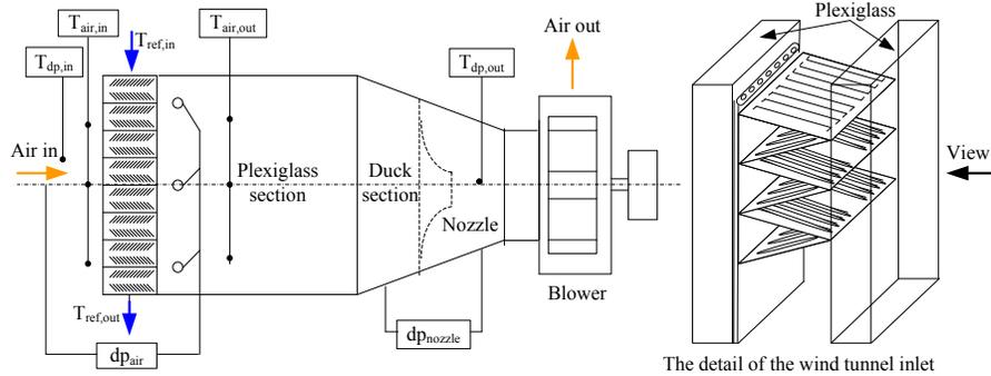
Figure 2: The open wind tunnel inside the environmental chamber
