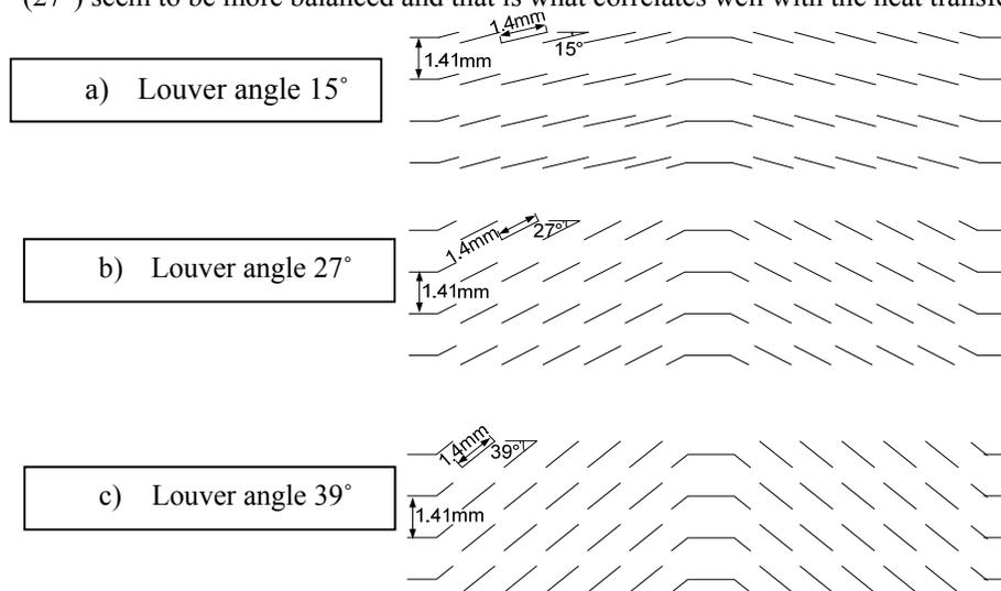
Fig. 5: Louvered-fin arrays for fin pitch 18 fpi (fin spacing 1.41mm), louver pitch 1.4 mm, louver angle  $15^\circ$ ,  $27^\circ$ ,  $39^\circ$
