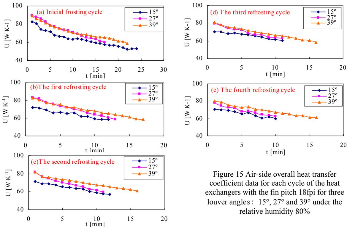
Figure 15 Air-side overall heat transfer coefficient data for each cycle of the heat exchangers with the fin pitch 18fpi for three louver angles: 15°, 27° and 39° under the relative humidity 80%
