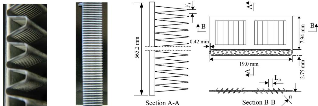
Figure 3: Structure of the test heat exchanger
