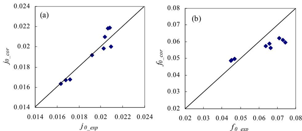
Fig. 7: Comparison of experimental data and correlations for the  $j_0$  and  $f_0$  factor
