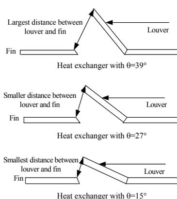
Figure 13: Drawings illustrating the impact of the louver angle on the channel area that is available for water to flow.
