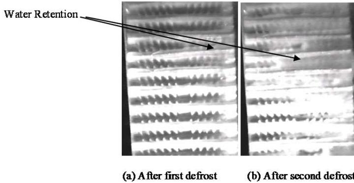
Figure 9: Visual observation of water retention after the first and second refrosting periods.
