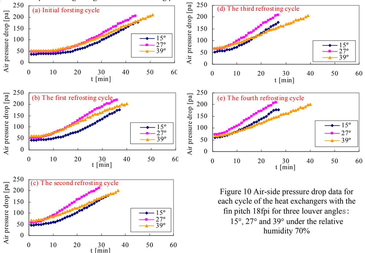
Figure 10 Air-side pressure drop data for each cycle of the heat exchangers with the fin pitch 18fpi for three louver angles: 15°, 27° and 39° under the relative humidity 70%
