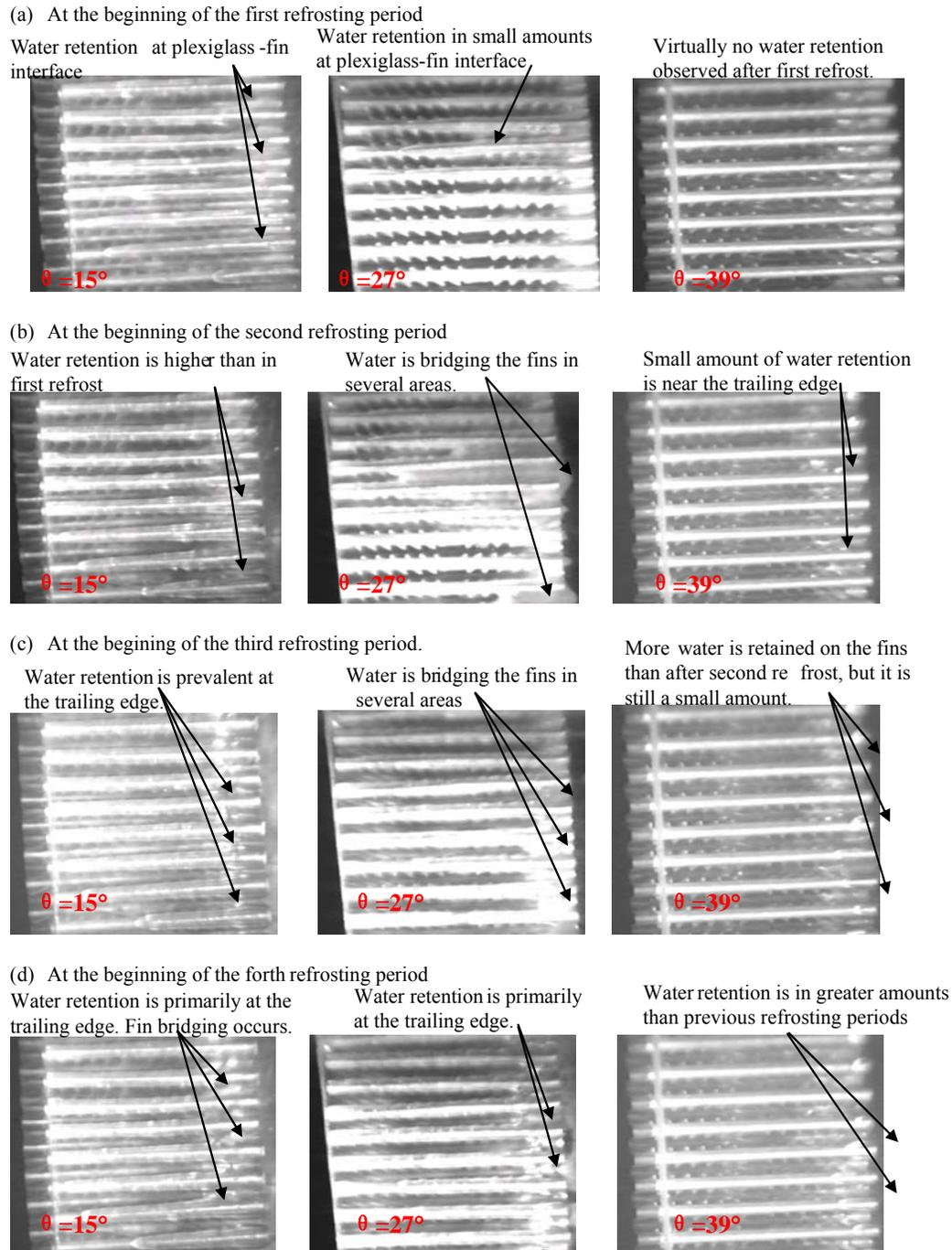
Figure 11: Heat exchangers with fin pitch 18fpi and louver angle 15°, 27° and 39° at beginning of refrost
