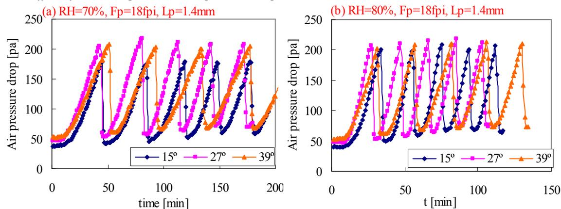
Figure 8: Effect of relative humidity on the air-side pressure drop for heat exchangers with louver angle  $15^\circ$ ,  $27^\circ$  and  $39^\circ$  for the fin pitch 18fpi during the first five frosting periods, face velocity: 3.5m/s
