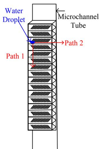
Figure 12: Illustration of water movement and removal modes.
