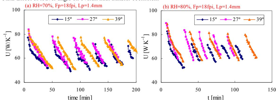
Figure 14: Effect of humidity on overall heat transfer coefficient for heat exchangers with louver angle 15°, 27° and 39° for the fin pitch 18fpi heat exchanger during the first five frosting periods
