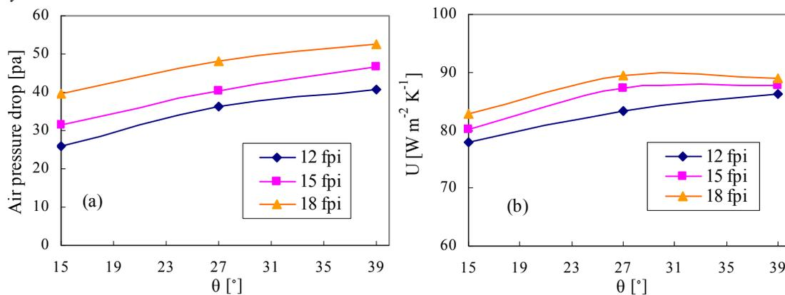
Fig. 4: Variations of air-side pressure drops and overall heat transfer coefficient with louver angle at the beginning of the first frosting cycle (clean surface) for three different fin pitches at face velocity: 3.5 m/s
