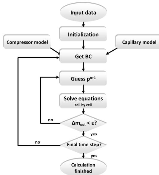
**Figure 1:** Information flow chart of the computation algorithm
