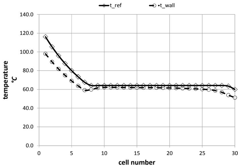
**Figure 5:** Temperature comparison: Condenser walls vs. refrigerant
