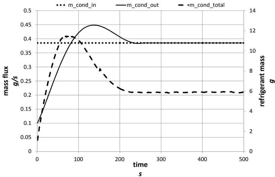
**Figure 2:** Mass fluxes entering and leaving the condenser and total refrigerant mass within the condenser
