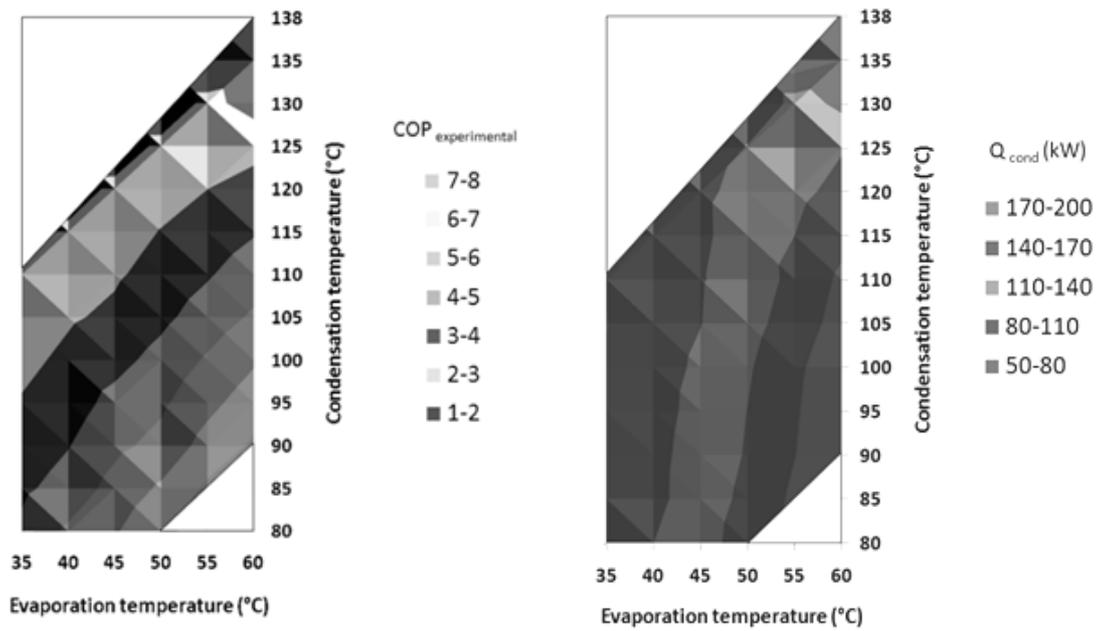
**Figure 7 :** (Left): HP COP and (right): delivered power at condenser (in kW) depending on evaporation and condensation temperature (in °C)
