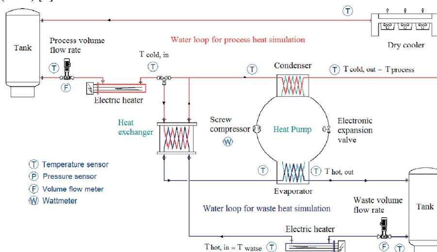
**Figure 4:** Scheme of the experimental set-up
