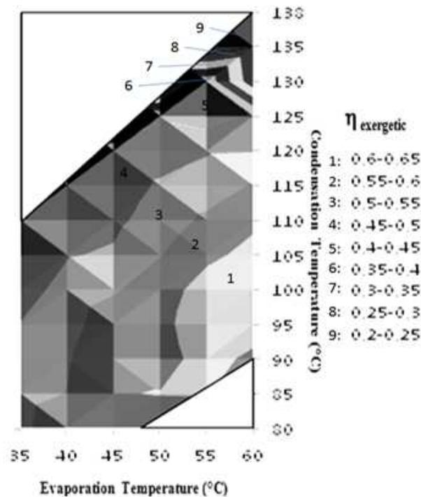
**Figure 8 :** diagram exegeretic efficiency depending evaporation and condensation temperature (in °C)
