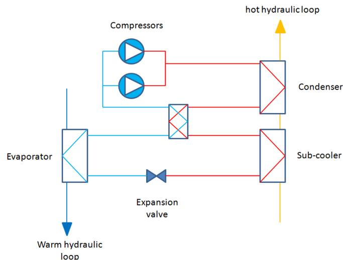
**Figure 5:** Scheme of the ALTER ECO heat pump
