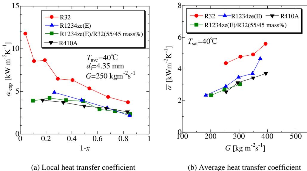
Figure 3: Condensation heat transfer coefficient
