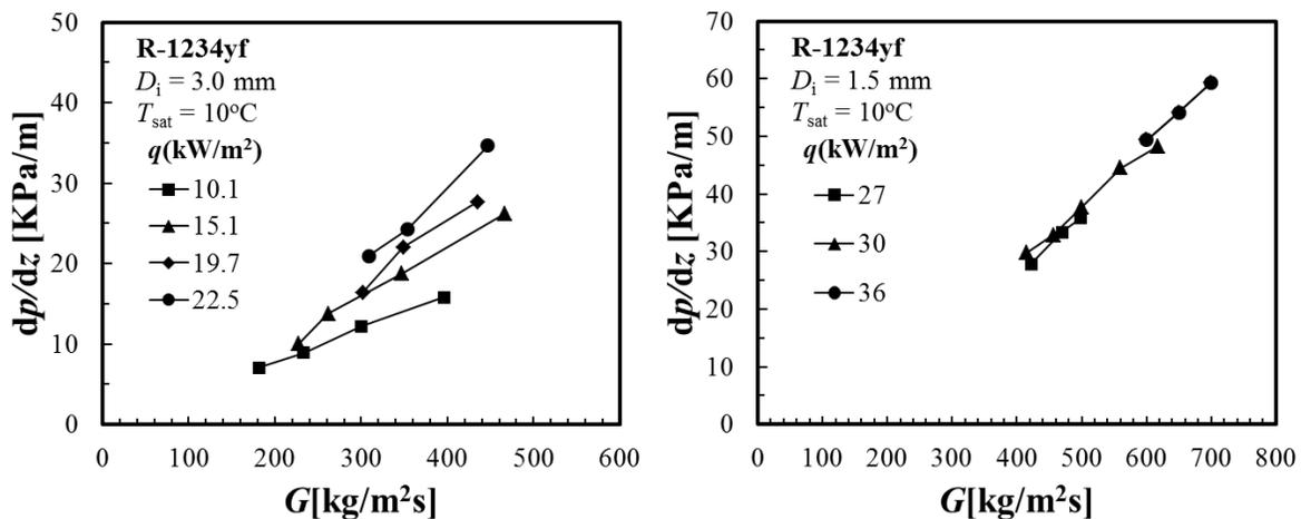
Figure 2 : The effect of mass flux and heat flux on pressure drop
