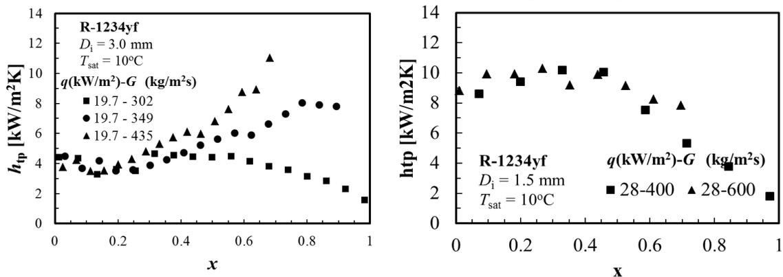
Figure 3 : The effect of mass flux on heat transfer coefficient.
