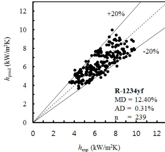
**Figure 7:** Heat transfer coefficient comparison between the present experimental data ( $h_{exp}$ ) and the prediction with the newly modified correlation ( $h_{pred}$ )
