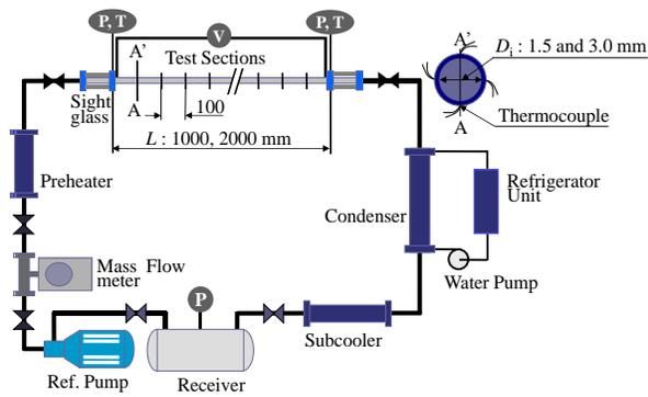
**Figure 1:** Experimental test facility
