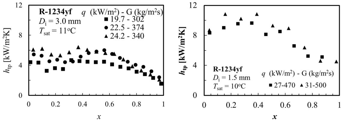
Figure 4 : The effect of heat flux on heat transfer coefficient.
