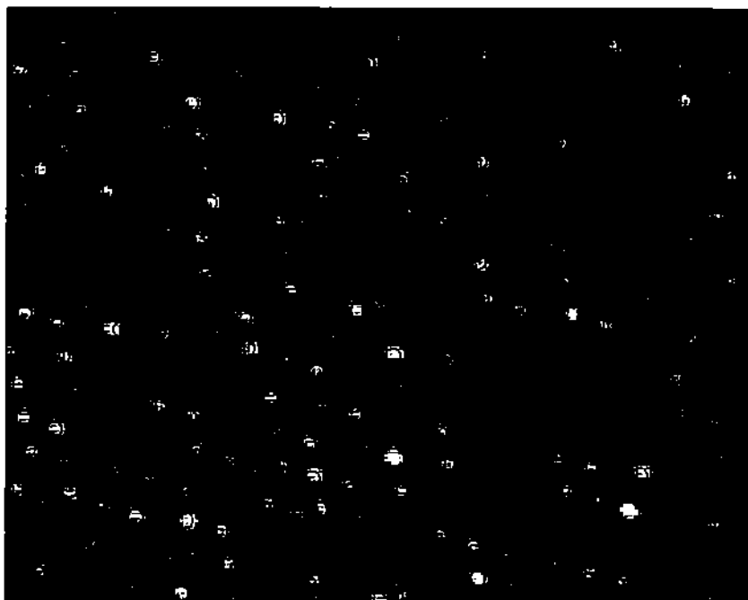
Figure 4: Peaks located with the depth-first search algorithm. The located peaks have been marked by small circles that delimit the zone of influence of each peak. Note that some of the peaks are located with poor accuracy.
