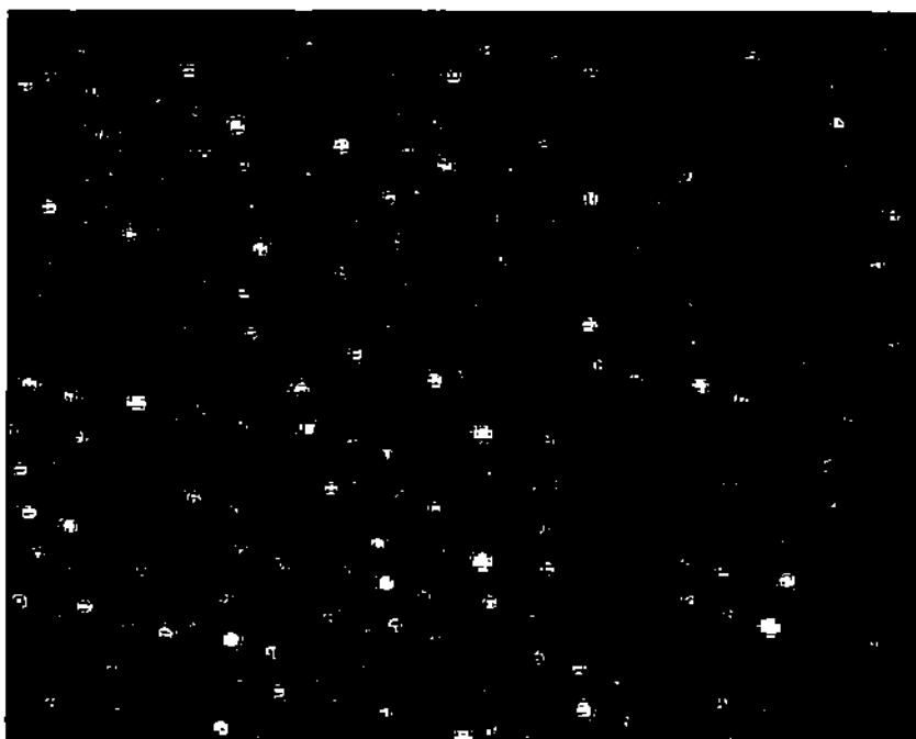
Figure 5: Peaks located with the dimension-reduction algorithm. Note the improvement over the DF algorithm in the accuracy of defining the zone of influence of each peak.
