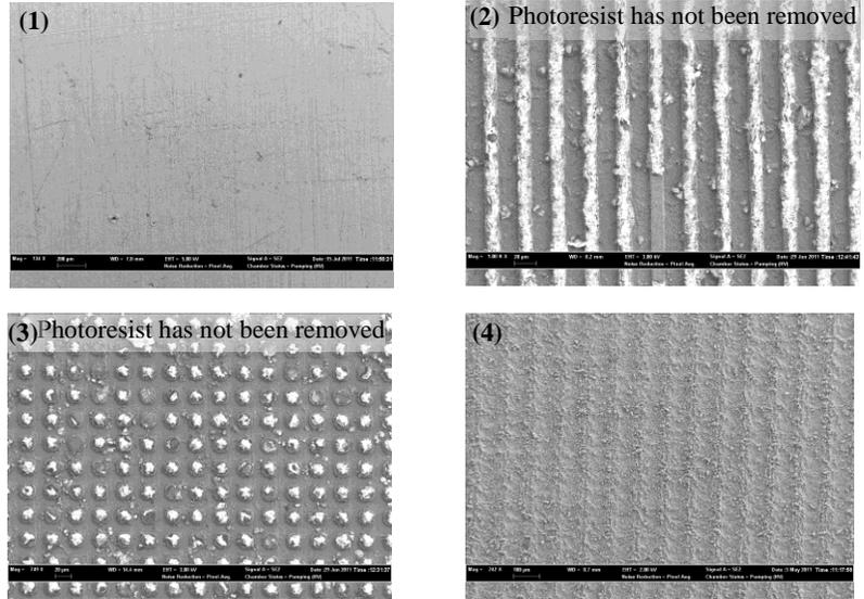
Figure 6: SEM images of prepared test surfaces— (1) baseline, (2) micro-channels, (3) micro posts, and (4) laser-etched micro channels
