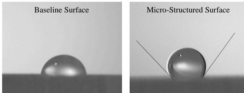
Figure 1: Image of a water droplet on a micro-structured aluminum surface and the impact of this surface structure on the contact angle
