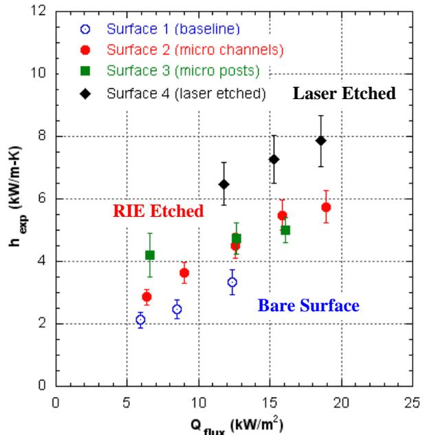
Figure 12: Comparison of Surface 4 versus the other surfaces reveals that it performed the best
