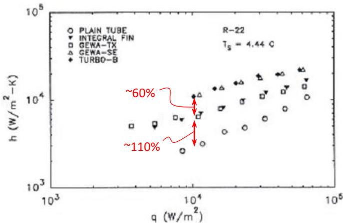
Figure 13: Heat transfer data for R-22 on commercially available enhanced surfaces (Webb, 1994)
