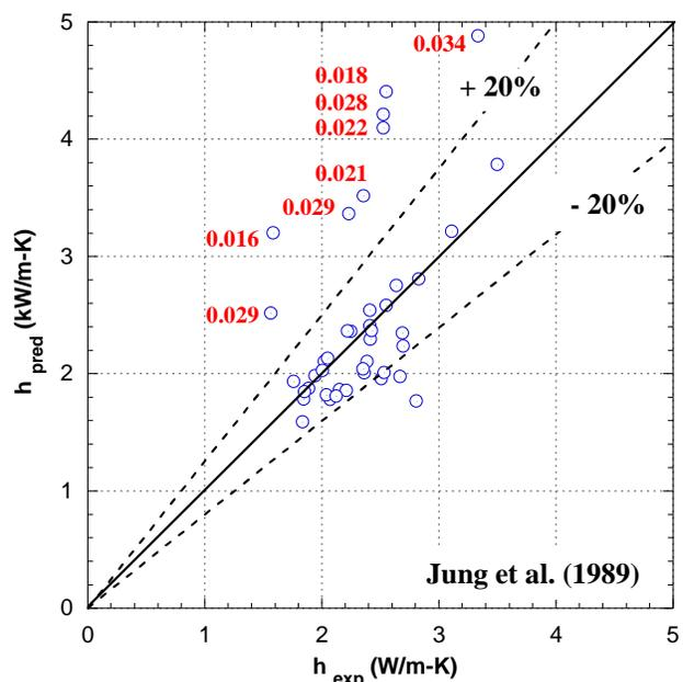
Figure 8: Comparison with Jung et al. (1989) model with vapor quality superimposed for cases of poor prediction
