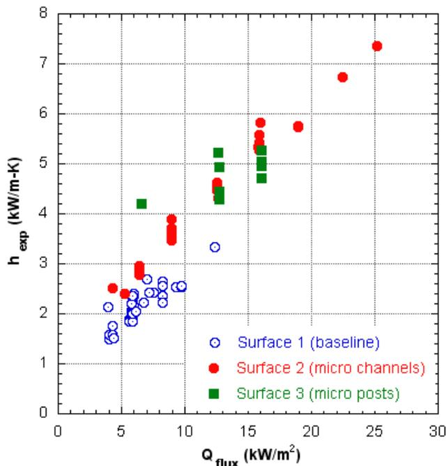
Figure 9: Experimental heat transfer coefficient versus applied heat flux for Surfaces 1, 2, and 3
