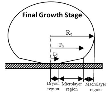
Figure 2: Final bubble growth stage (Zhao et al., 2002)
