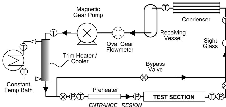
Figure 3: Schematic of the two-phase convective flow boiling test loop
