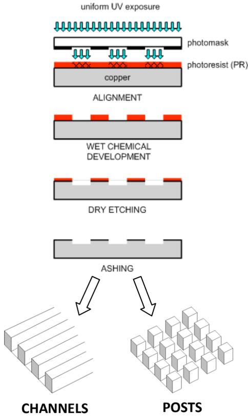
Figure 5: Photolithographic procedure used to prepare Surfaces 1-3
