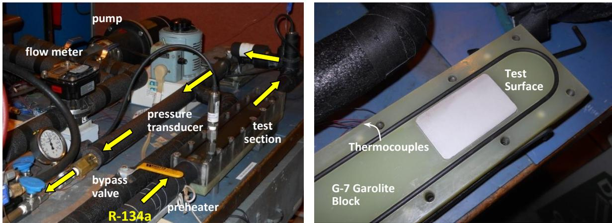
Figure 4: Pictures of the constructed flow boiling test loop
