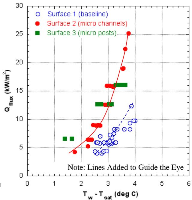
Figure 10: Applied heat flux versus wall superheat for Surfaces 1, 2, and 3
