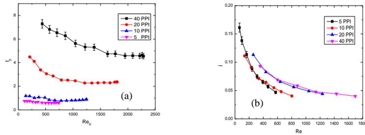
**Figure 9:** Thermal-hydraulic performance in terms of the conventional length scale, (a) friction factor, (b) Colburn  $j$  factor.
