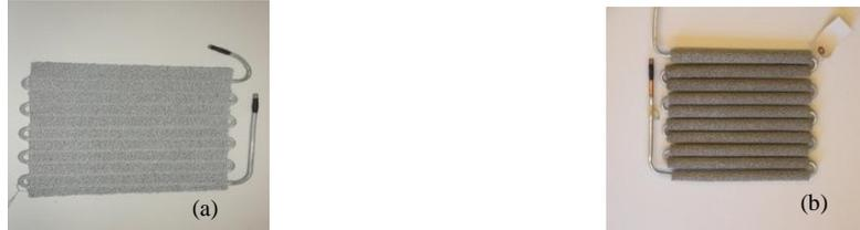
**Figure 3:** Metal foam heat exchangers with different geometry (a) Sample 1-continuous block (b) Sample 2-Annular
