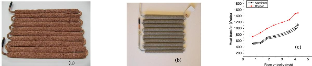
Figure 7: Metal foam heat exchangers with different base material, (a) copper and (b) aluminum, and (c) their heat transfer rates
