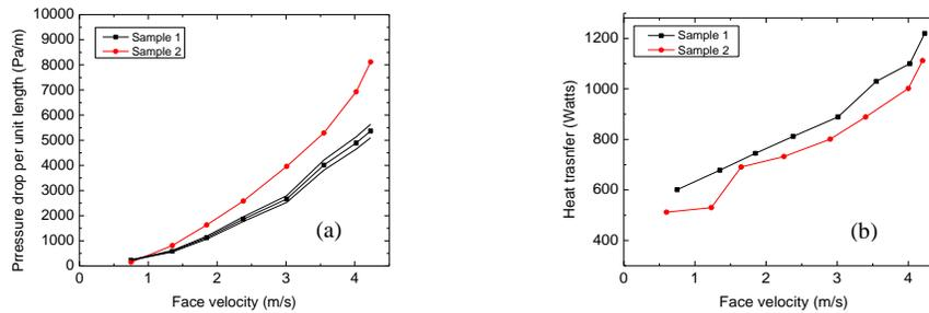
**Figure 4:** Pressure drop per unit length for foams of different geometry
