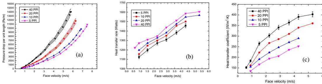
**Figure 2:** Thermal-hydraulic data for aluminum metal foams (a) pressure gradient, (b) heat duty, (c) heat transfer coefficient.
