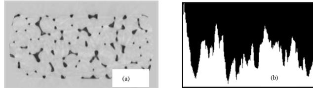
**Figure 8:** Image processing for cross sectional view of 5 PPI metal foam (a) X-rays image of foam slice (b) intensity distribution of the image.
