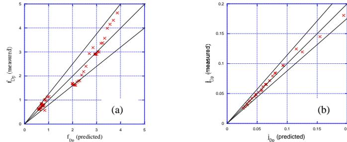
**Figure 10:** Thermal-hydraulic performance in terms of the alternative length scales from Equations (16) and (17), (a) friction factor, (b) Colburn  $j$  factor.
