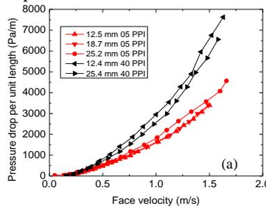
Figure 5: Flow depth effects on pressure gradient
