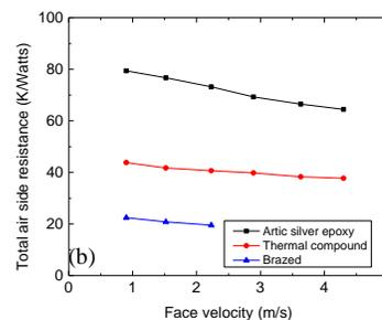
Figure 6: Bonding effects on air-side thermal resistance
