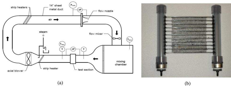
**Figure 1:** (a) Wind tunnel apparatus, (b) flat tube metal foam heat exchanger (10 PPI metal foam)
