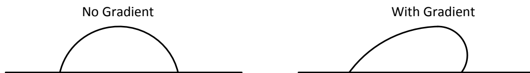
Fig. 2 Schematic of a droplet on a (a) homogeneous surface, and (b) a surface with an underlying gradient
