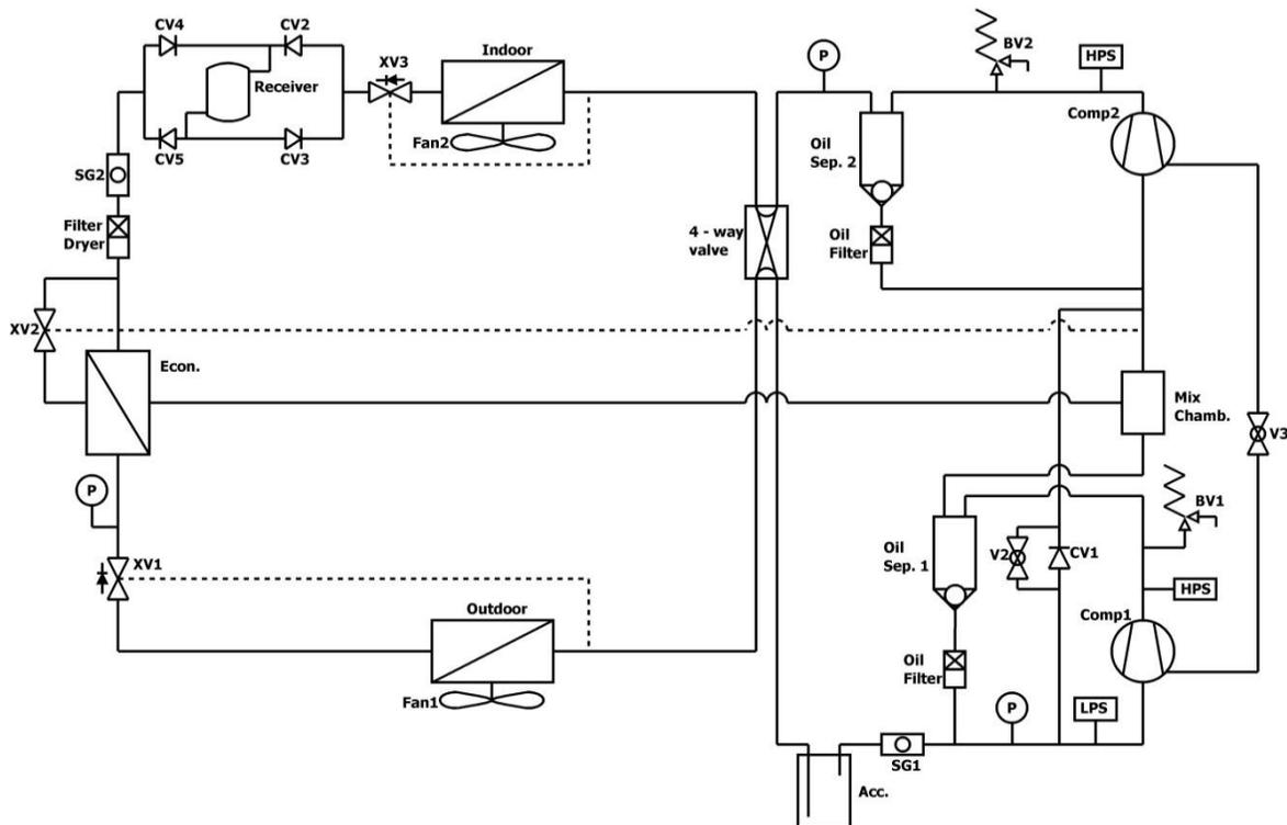
**Figure 1:** Piping schematic of 2-stage air-source heat pump with economizing and low-side compressor bypass
