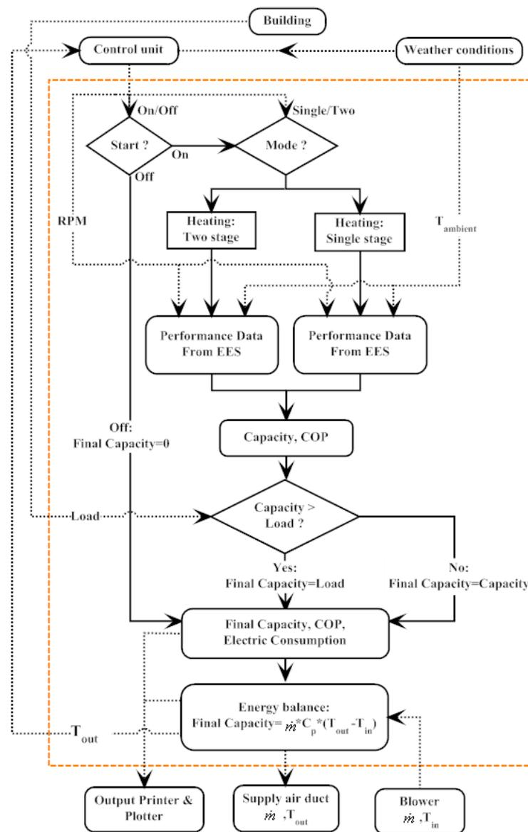
**Figure 7:** Cold climate heat pump logic for the module developed within TRNSYS
