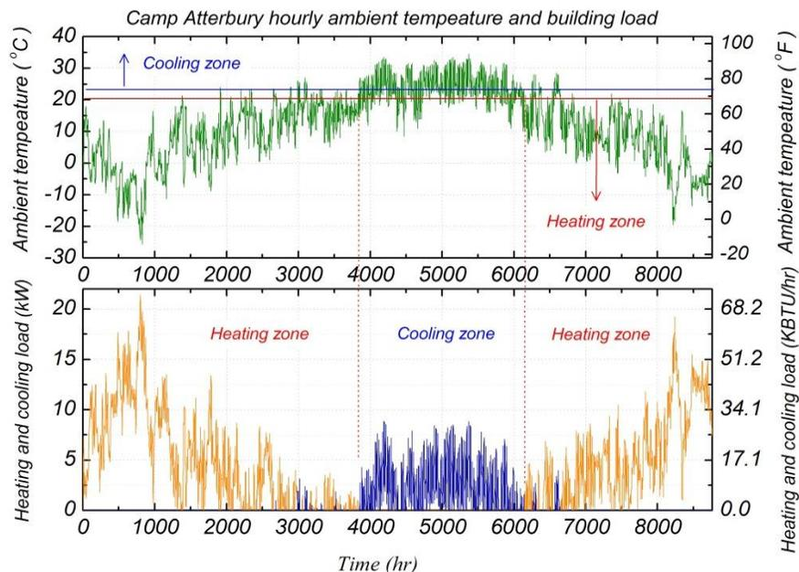
**Figure 8:** Ambient temperature and cooling or heating load at the military barracks
