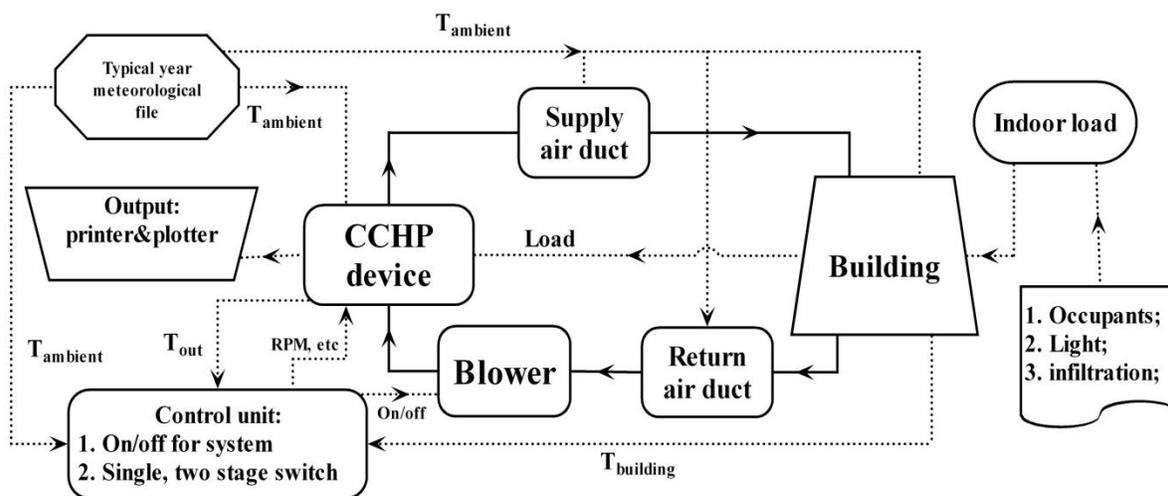
**Figure 4:** TRNSYS model layout
