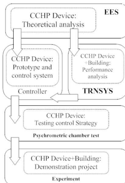
**Figure 2:** How simulation results are utilized for the field demonstration
