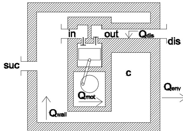
**Figure 3:** Simplified scheme of a hermetic compressor
