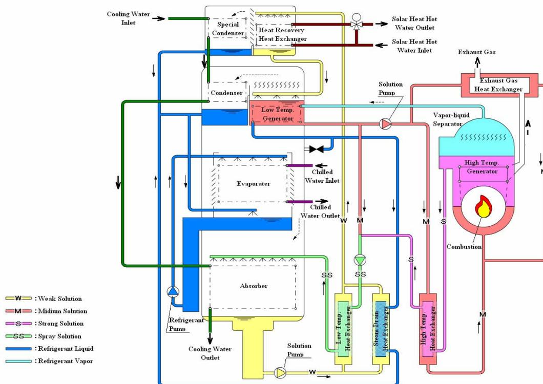
Fig. 2: Cooling cycle flow of Solar-Driven Hybrid Chiller
