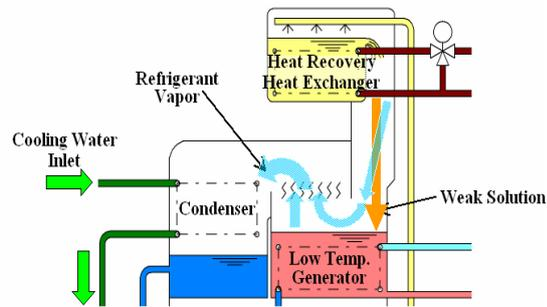
Fig. 4: Principle of Solar-Driven Hybrid Chiller
