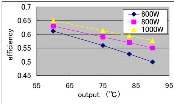
Fig. 8: Heat collection efficiency of Solar collector
