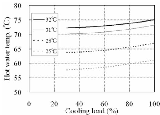
Fig. 5: Hot water temperature for which Solar-Driven Hybrid Chiller can be used
