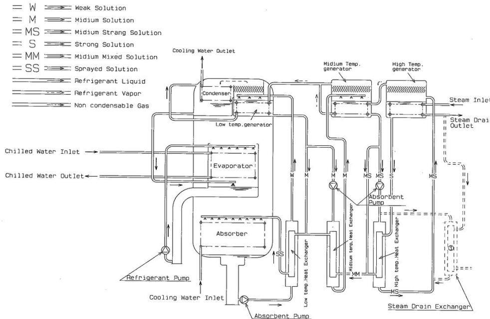
Fig. 5 Cycle flow of steam-fired triple effect absorption chiller.
