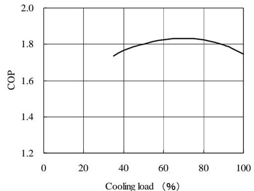
**Fig. 4 Partial load characteristics of triple effect absorption solar cooling system**
