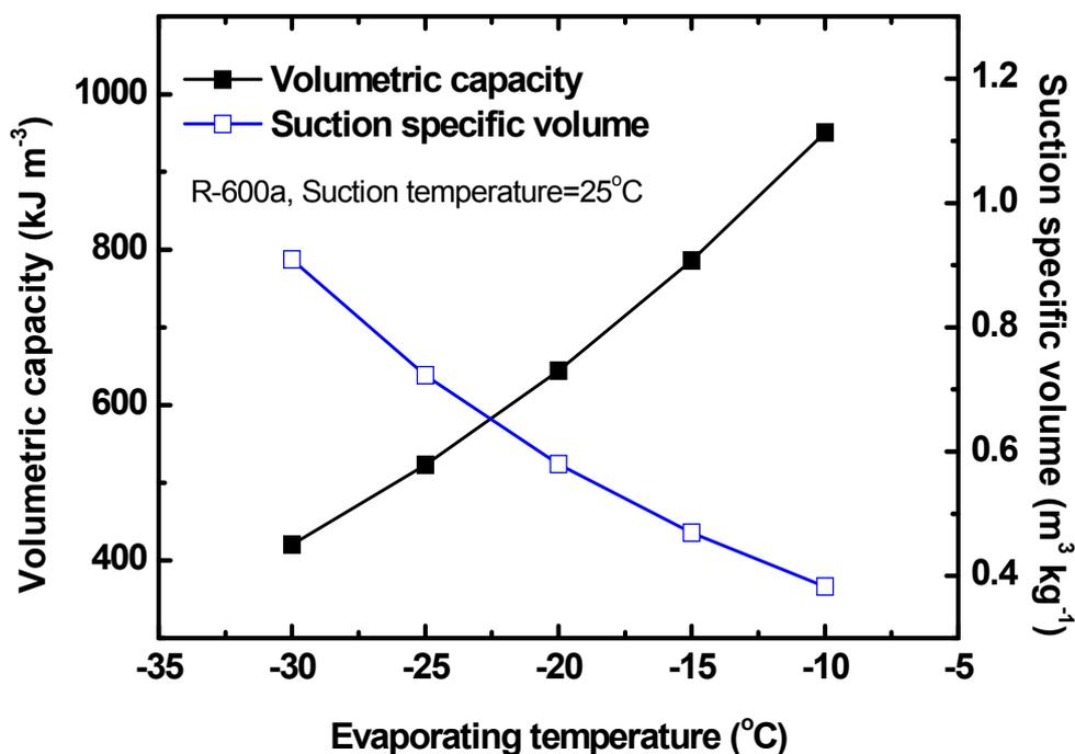
**Figure 2:** Variations of the volumetric capacity and suction specific volume of R-600a
