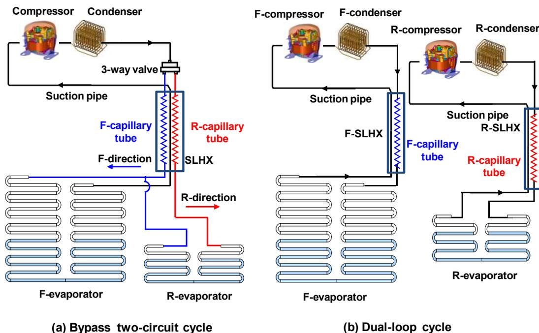
Figure 1: Schematic diagrams of the bypass two-circuit cycle and the dual-loop cycle
