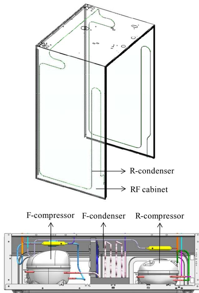
**Figure 3:** R-condenser attached onto the RF cabinet and the redesigned machine room
