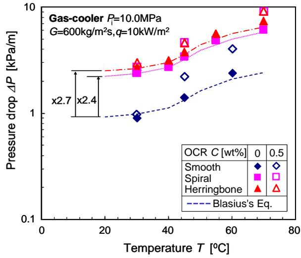
Figure 5: Effect of temperature on pressure drop in gas cooler condition.
