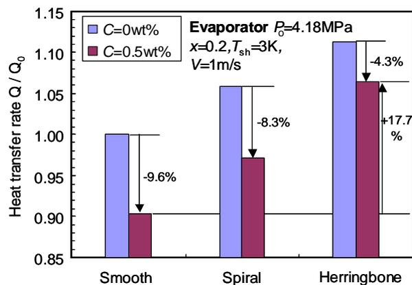
**Figure 10:** Results of heat transfer rate with and without PAG oil for each tube in evaporator.
