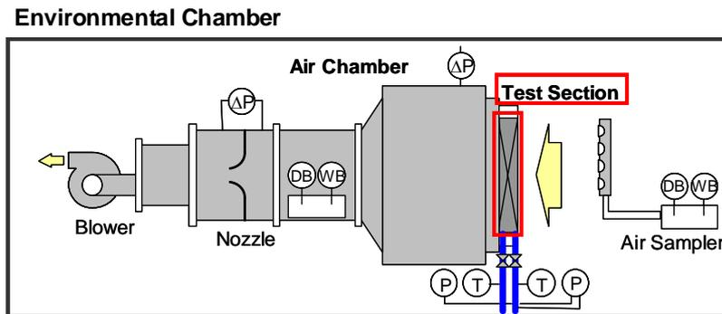
Figure 3: Schematic diagram of the test section (Experiments using heat exchangers).
