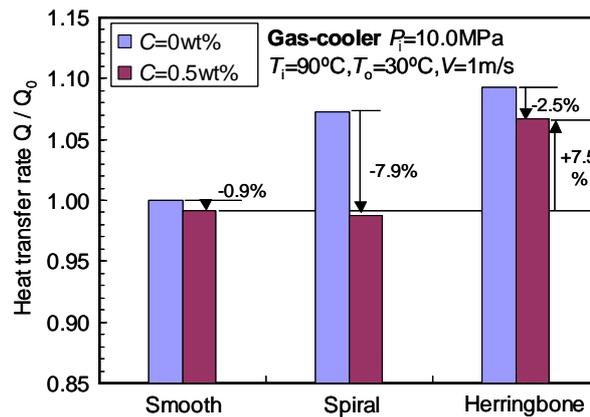
**Figure 9:** Results of heat transfer rate with and without PAG oil for each tube in gas cooler.
