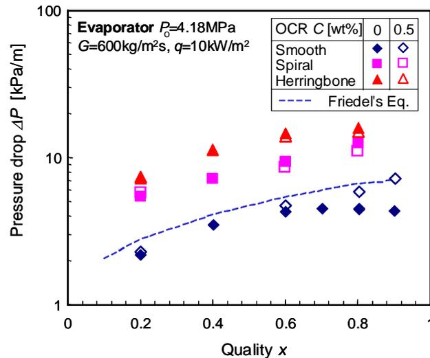
Figure 7: Effect of quality on pressure drop in evaporator condition.
