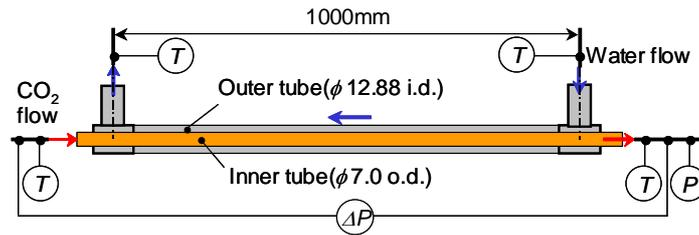
Figure 2: Schematic diagram of the test section (Experiment using double pipe heat exchangers).
