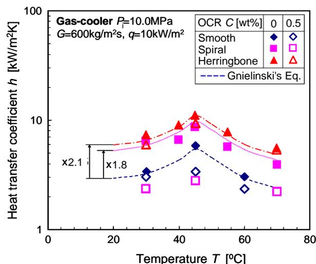
Figure 4: Effect of temperature on heat transfer coefficient in gas cooler condition.
