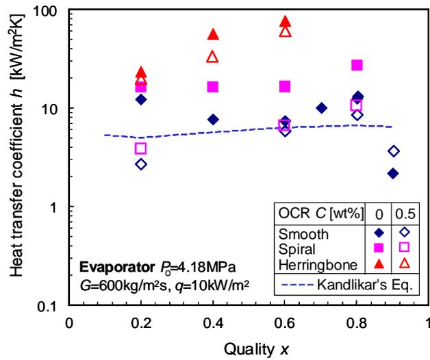
Figure 6: Effect of quality on heat transfer coefficient in evaporator condition.
