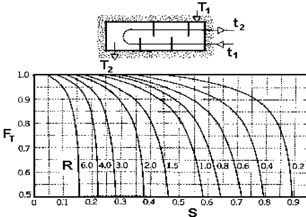
Figure 5: F factor in function of dimensionless ratios S and R.
