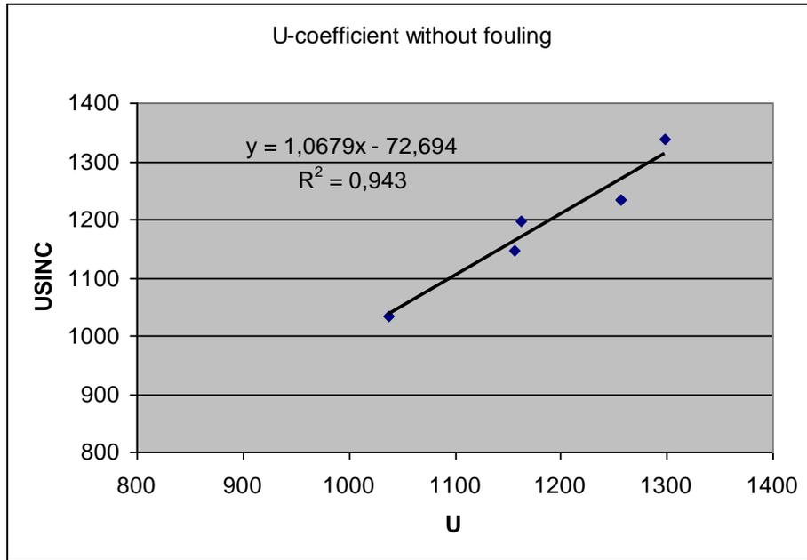
Figure 10: Overall heat transfer coefficient (without fouling, Usinc) compared with the theoretical value obtained by mass balance in the heat exchanger (U)
