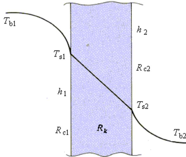
Figure 1: temperature profile through a wall between two fluids
