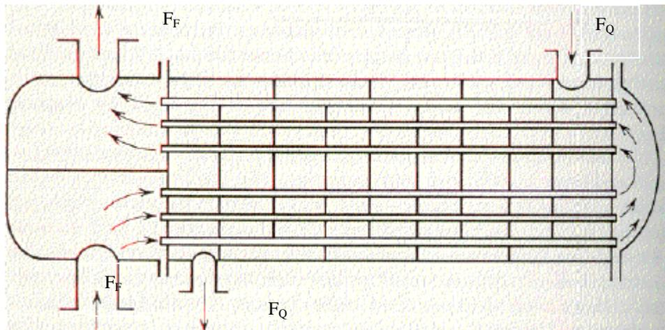
Figure 6: Heat exchanger shell and tube type
