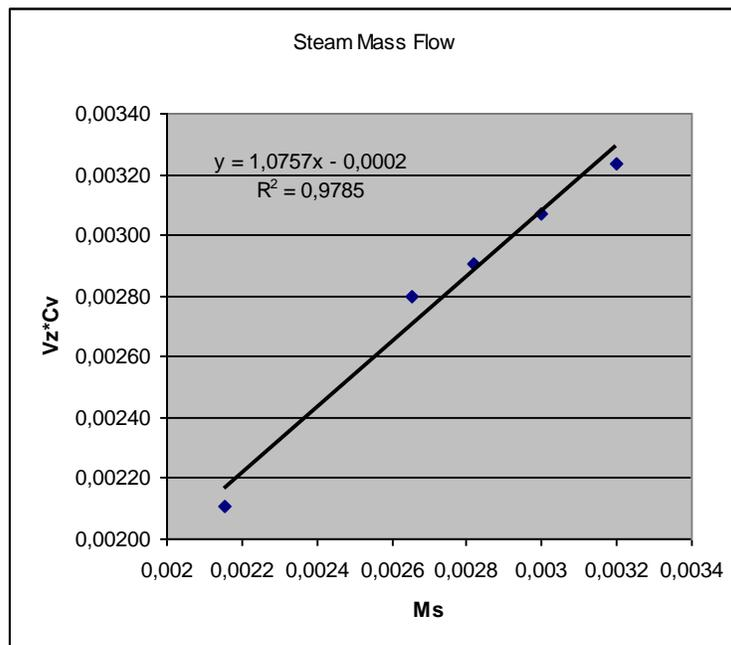
Figure 11: Correlation measuring the mass flow ( $V_z$ ) compared with the value obtained by the mass balance in the heat exchanger ( $M_s$ )
