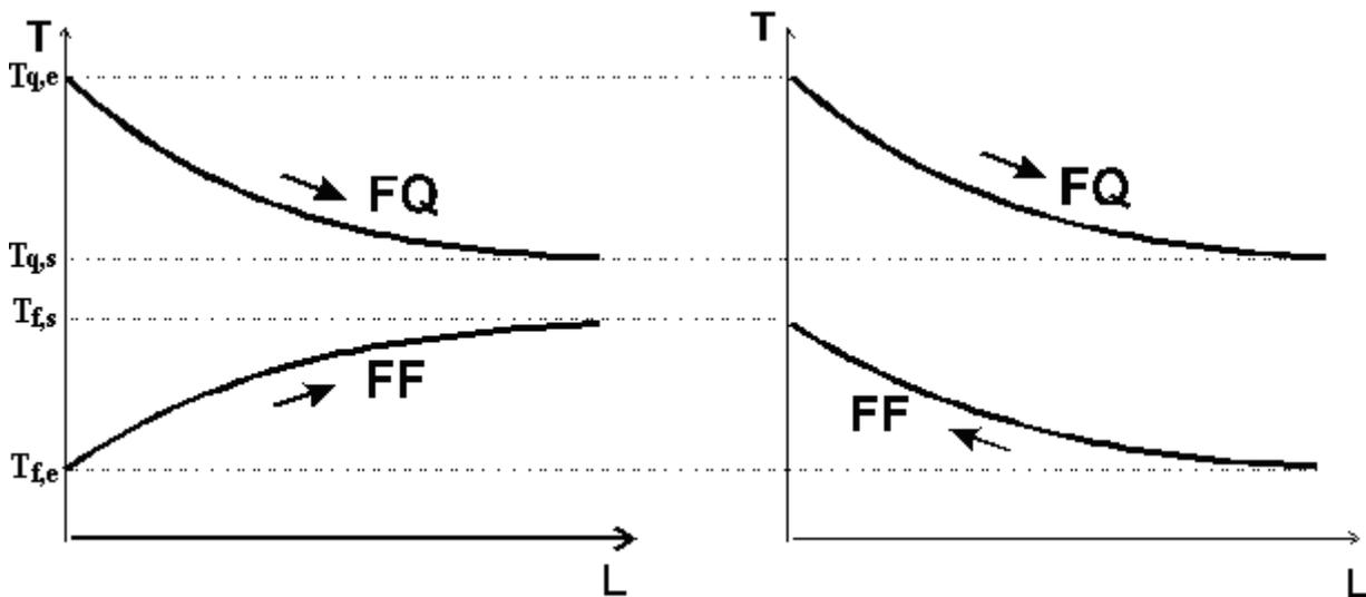
Figure 4: Configuration of heat exchangers for calculating the  $\Delta TML$ .
