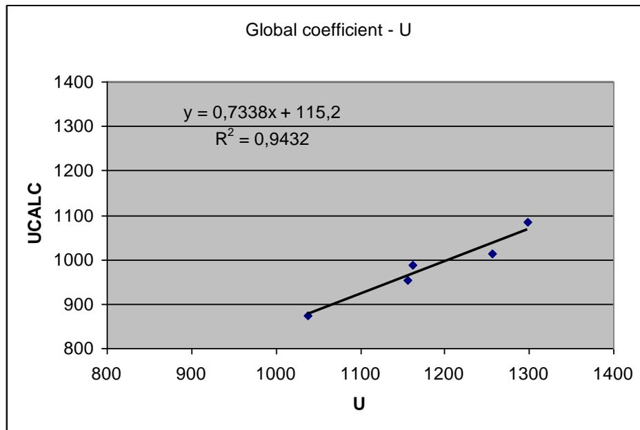
Figure 9: Overall heat transfer coefficient (Ucalc) compared with the theoretical value obtained by mass balance in the heat exchanger (U)
