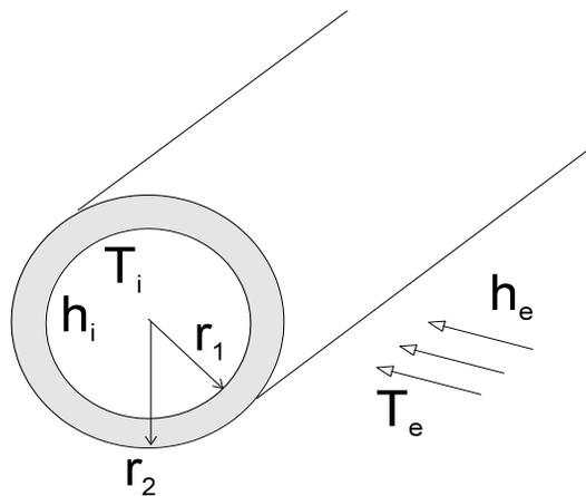
Figure 3: thermal resistance due to conduction and convection.
