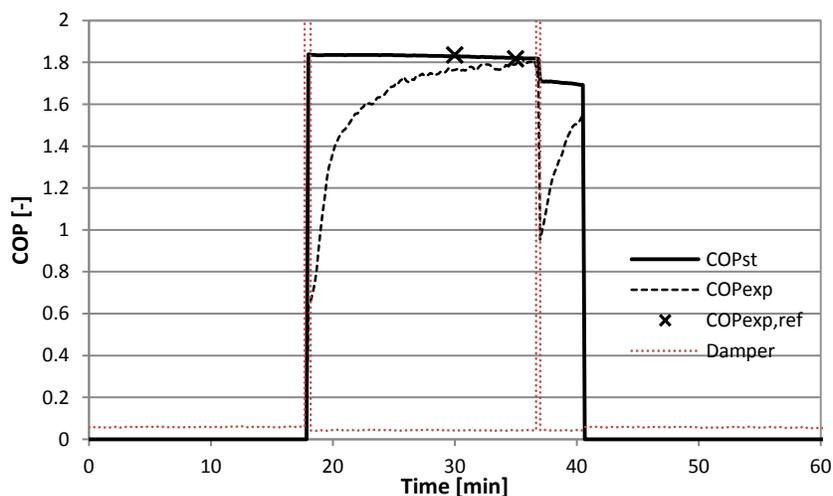
Figure 4: Comparison of steady-state  $COP_{st}$  and experimental  $COP_{exp}$ .
