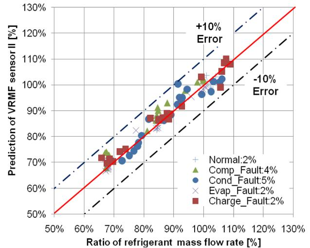
**Figure 4: Performance of VRMF sensor II based on energy balance for system I under no fault and fault conditions (RMS of errors shown for each fault type)**
