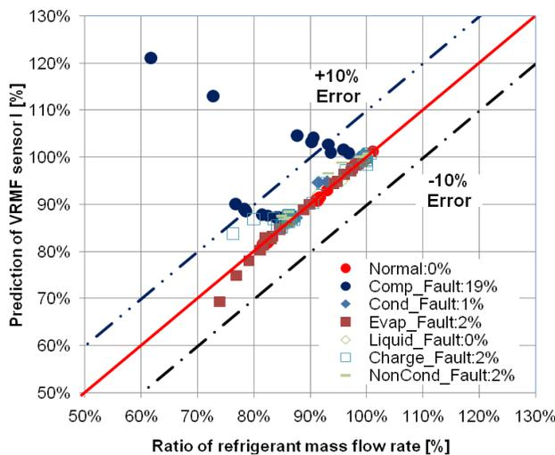
**Figure 1: Performance of VRMF sensor based on fixed-speed compressor map for system III under no fault and fault conditions (RMS of sensor errors shown for each fault type)**
