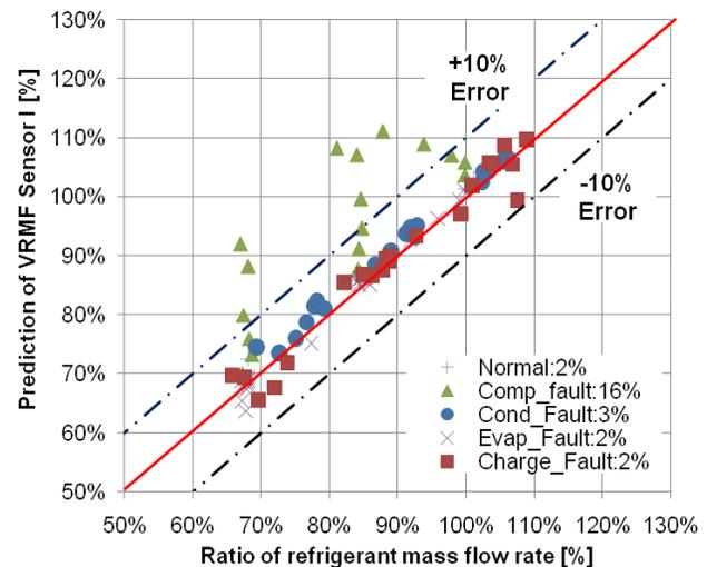
**Figure 2: Performance of VRMF sensor based on variable speed compressor map for system I under no fault and fault conditions (RMS of sensor errors shown for each fault type)**
