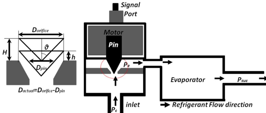
Figure 8: Flow passage structure and geometric models for EEV
