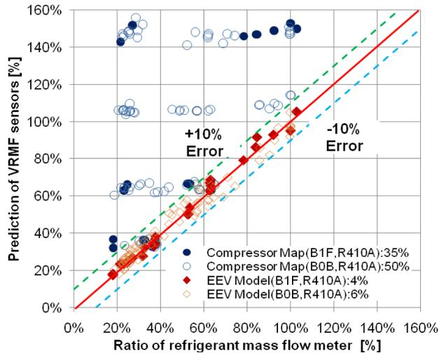
**Figure 13: Comparison of VRMF sensor outputs for system II (R410A) with compressor flow fault**
