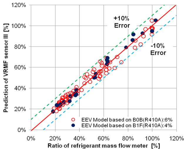
**Figure 9: Performance of VRMF sensor III based on EEV with R410a as refrigerant for system II**
