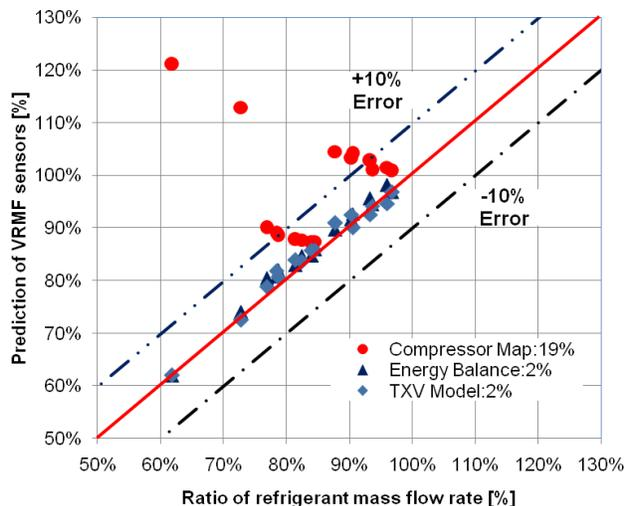
**Figure 11: Comparison of VRMF sensor outputs for system III with compressor flow fault**
