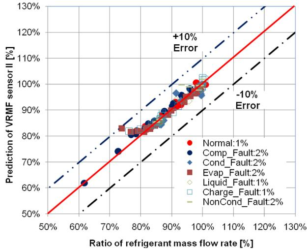
**Figure 3: Performance of VRMF sensor II based on energy balance for system III under no fault and fault conditions (RMS of errors shown for each fault type)**
