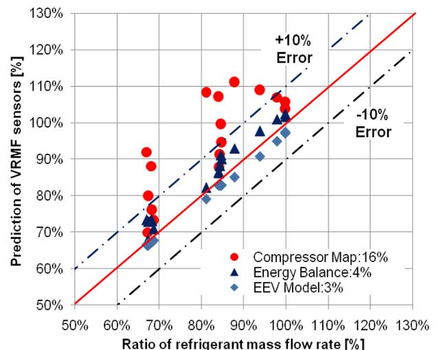
**Figure 12: Comparison of VRMF sensor outputs for system I with compressor flow fault**
