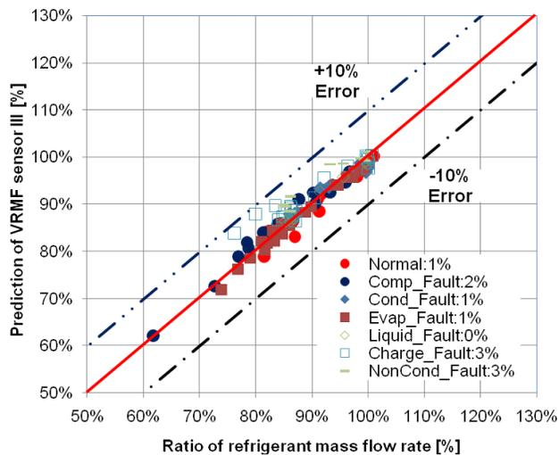
**Figure 6: Performance of VRMF sensor III based on TXV for system III under no fault and fault conditions (RMS of sensor errors shown for each fault type)**
