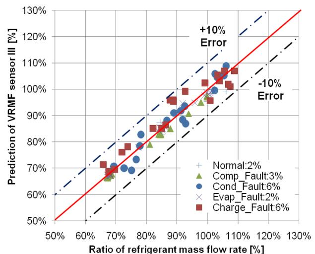
**Figure 7: Performance of VRMF sensor III based on EEV for system I under no fault and fault conditions (RMS of sensor errors shown for each fault type)**
