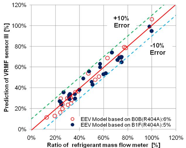
**Figure 10: Performance of VRMF sensor III based on EEV with R410a as refrigerant for system II**
