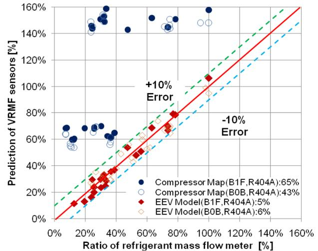
**Figure 14: Comparison of VRMF sensor outputs for system II (R404A) with compressor flow fault**
