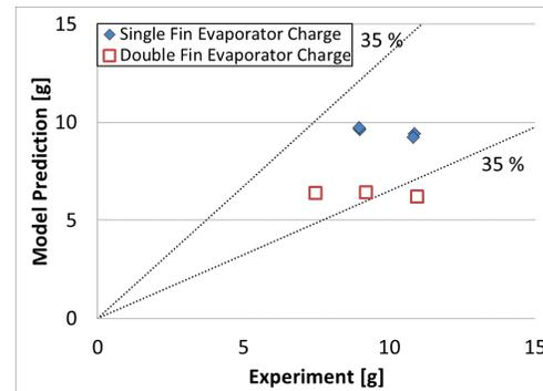
**Figure 6:** Charge prediction of serpentine evaporators using Graham (1997) void fraction correlation
