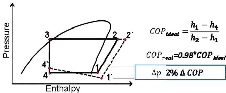
**Figure 7:** Comparison criteria for microchannel heat exchangers based on pressure drop that causes 2% change in COP
