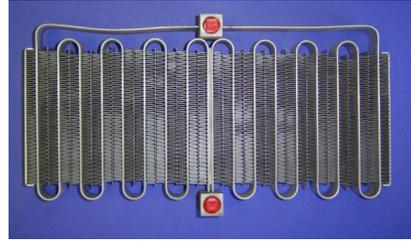
**Figure 4:** Double fin serpentine design evaporator from Hrnjak and Traeger (2005)
