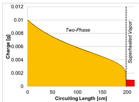
**Figure 1:** Charge distribution along serpentine evaporator with R290 from Traeger and Hrnjak (2005) shown in Fig. 3
