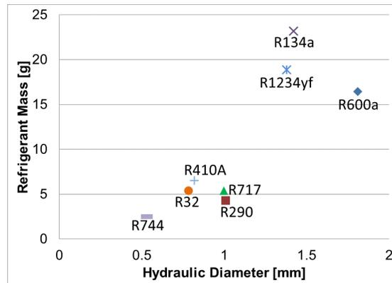
**Figure 11:** Refrigerant charge (Mass) and hydraulic diameter of serpentine evaporator for 1kW refrigeration system causing 2% difference from ideal COP due to evaporator pressure drop
