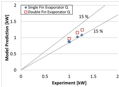
**Figure 5:** Capacity of serpentine evaporators using Pamitran et. al. (2009) and Park and Jacobi (2009)
