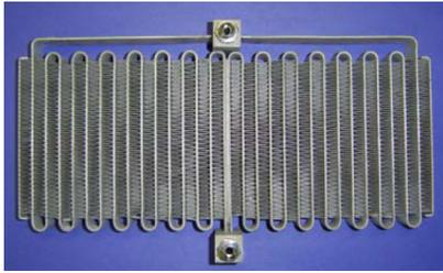
**Figure 3:** Single fin serpentine design evaporator from Hrnjak and Traeger (2005)
