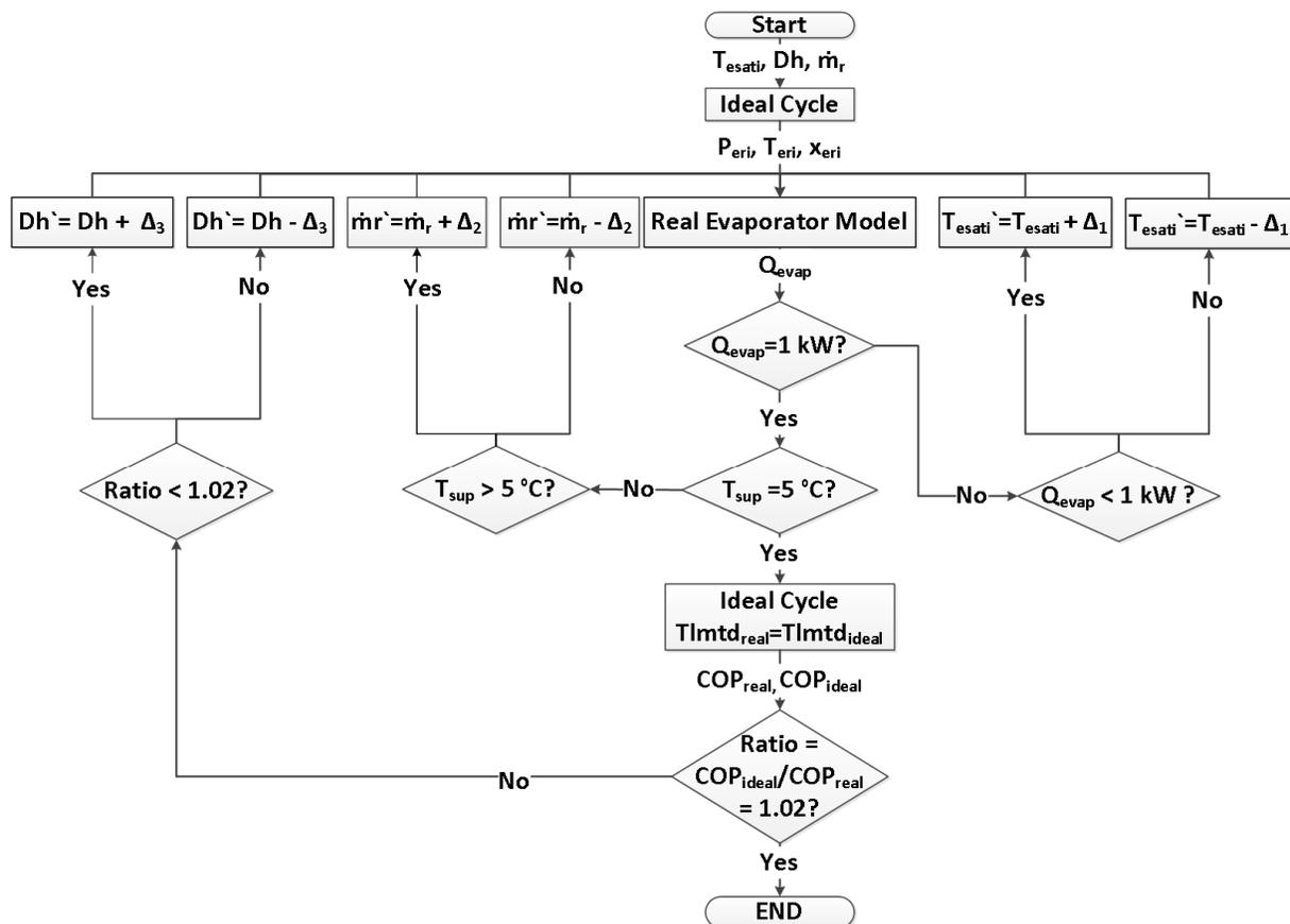
**Figure 10:** Logic flow diagram used to obtain 2% COP decrease due to pressure drop
