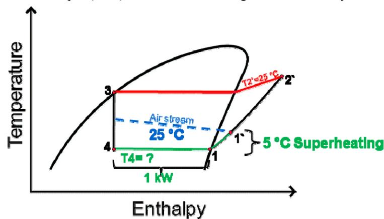
**Figure 8:** Air side and refrigerant side operating conditions for this example
