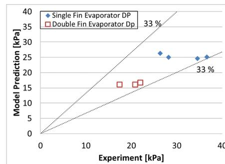
**Figure 2:** Souza and Mattos Pimenta (1995) correlation predicts R290 evaporators  $\Delta P$  data within 33 %
