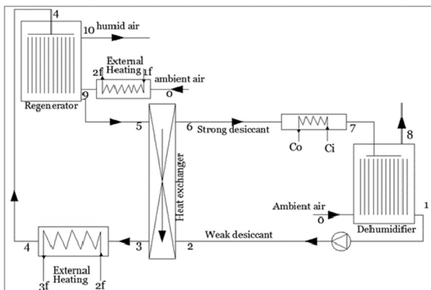
Figure 1: Schematic drawing of the liquid desiccant system
