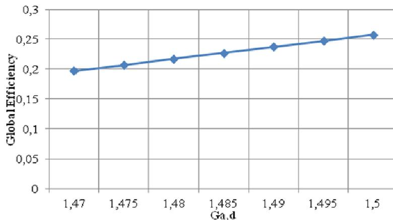
**Figure 7:** Influence of the dehumidifier air specific flow on the global exergy efficiency
