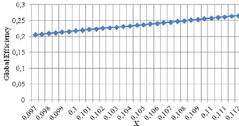
**Figure 8:** Influence of the dehumidifier inlet desiccant concentration on the global exergy efficiency
