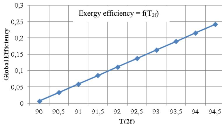
**Figure 4:** Influence of the hot flow temperature at the end of heat exchange with the regenerator inlet air on the global exergy efficiency
