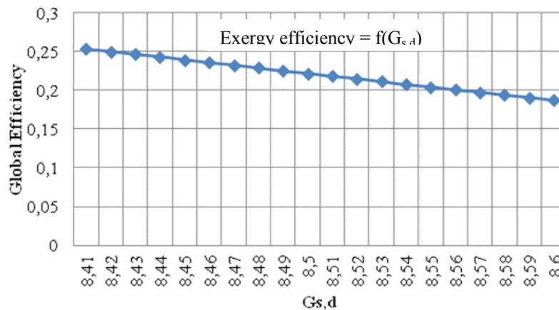
**Figure 6:** Influence of the dehumidifier desiccant specific flow on the global exergy efficiency
