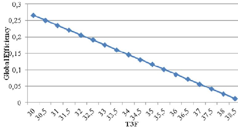
**Figure 5:** Influence of the hot flow temperature at the end of heat exchange with the weak desiccant on the global exergy efficiency
