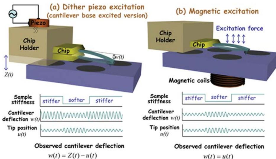
FIG. 1. (Color online) (a), (b) Schematics of force modulation AFM using magnetic and dither piezo excitation and corresponding waveforms (sample stiffness, cantilever deflection, and tip position).
