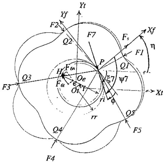
Fig. 1 All contact forces acting on the rotor & pinion
