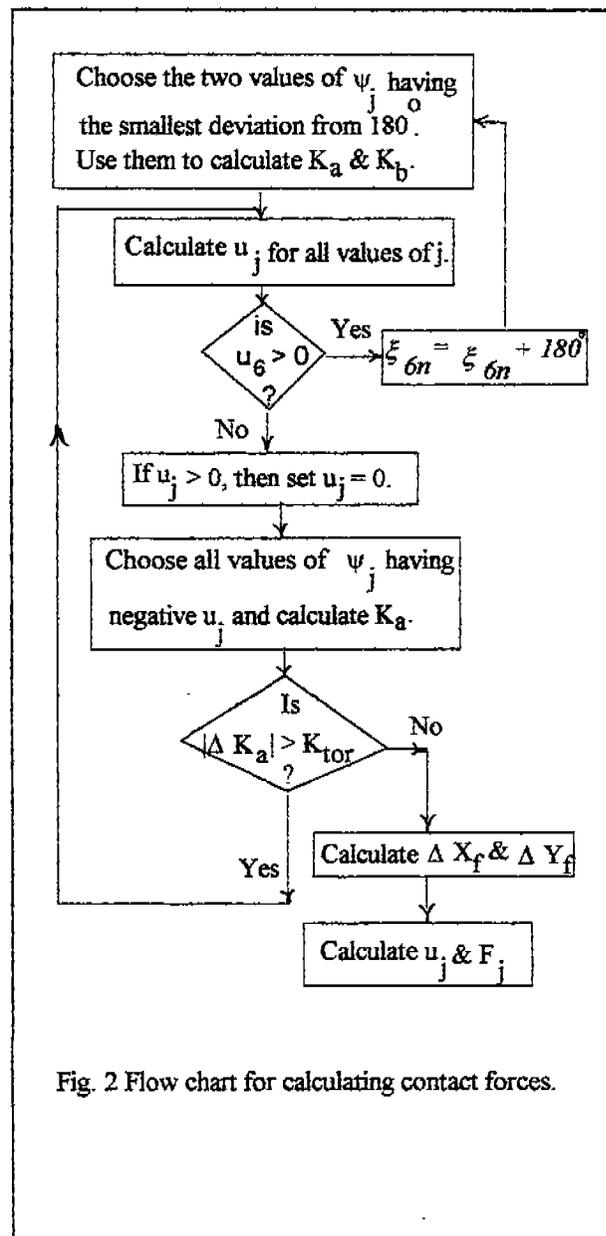
Fig. 2 Flow chart for calculating contact forces.
