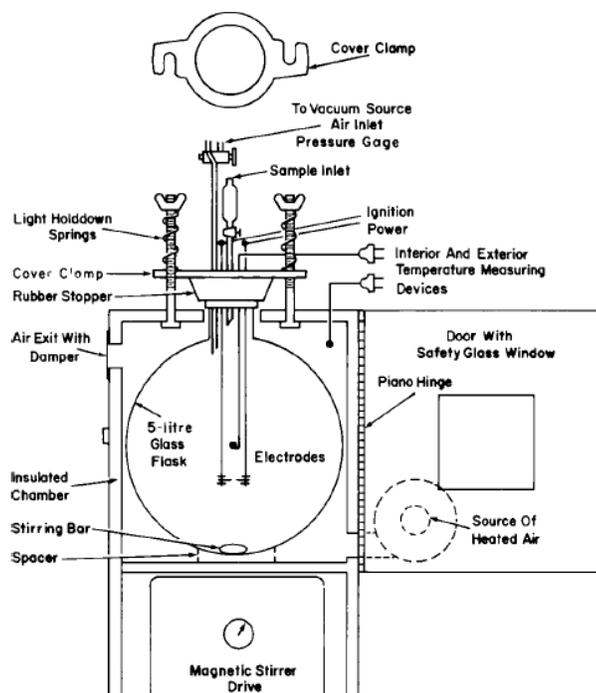
**Fig 1:** Apparatus for testing combustible gases or vapors
