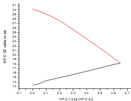
Fig 5: Flammability limit of HFC-134a/HFC-32 with PAG
