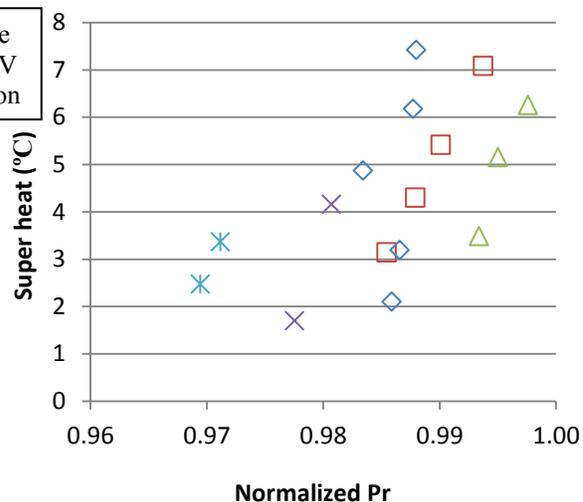
**Figure 5:** Superheat vs. Pressure ratio for DR-5 TXV optimization at AHRI A cooling conditions
