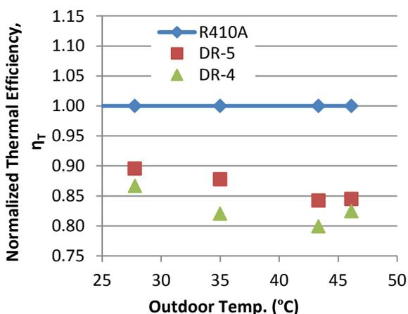
Figure 14: Thermal Efficiency (Drop-in test)
