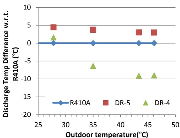
Figure 10: Discharge Temperature (Drop-in tests)
