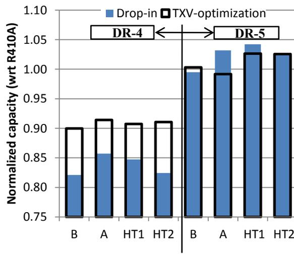
Figure 9: System capacity in TXV soft optimization for DR-4 and DR-5
