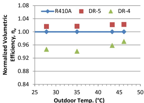
Figure 12: Volumetric Efficiency (Drop-in test)
