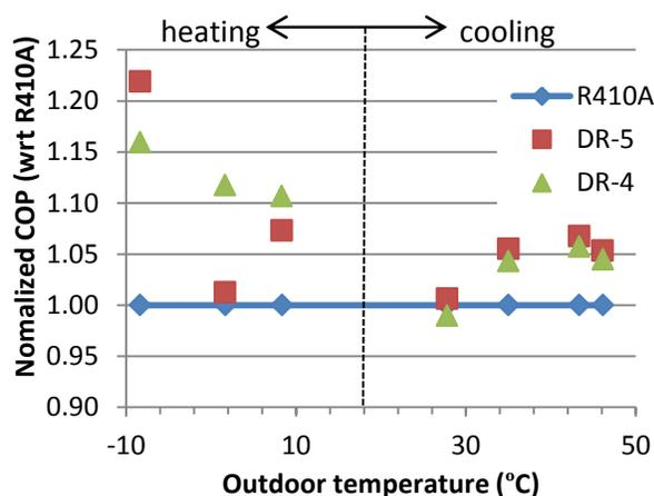
Figure 6: System performance in drop-in testing
