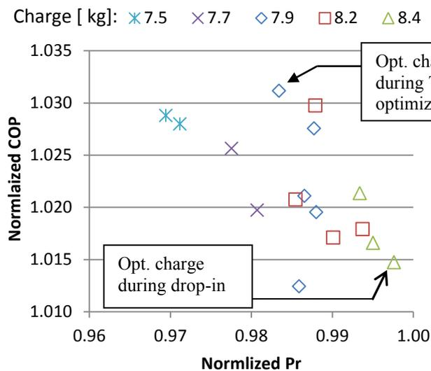
**Figure 4:** COP vs. Pressure ratio for DR-5 TXV optimization at AHRI A cooling conditions
