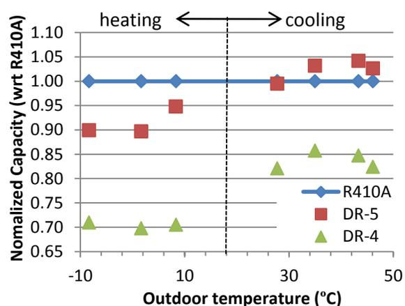
Figure 7: System capacity in drop-in testing
