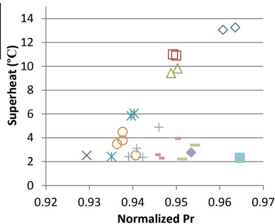
**Figure 3:** Superheat vs. Pressure ratio for DR-4 TXV optimization at AHRI A cooling conditions
