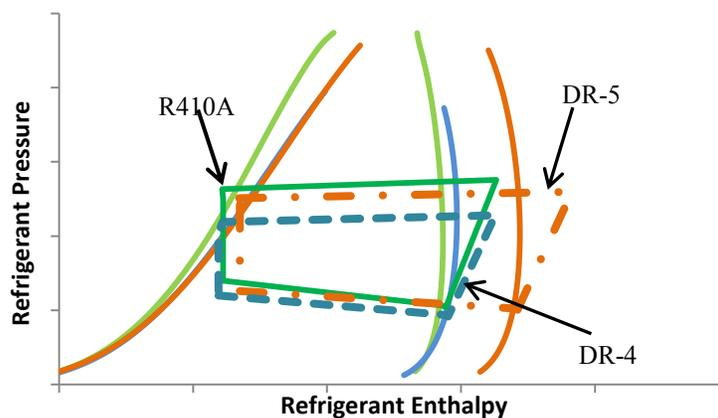
**Figure 1:** Schematic of the *P-h* diagrams for R410A, DR-4 and DR-5 during drop-in tests at AHRI A cooling conditions
