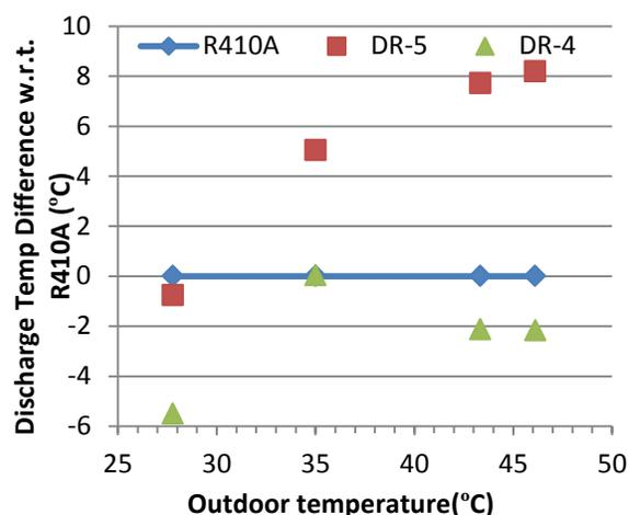
Figure 11: Discharge Temperature (TXV-optimization tests)
