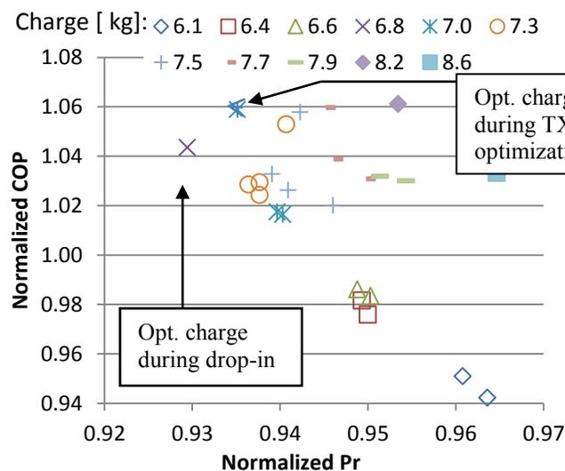
**Figure 2:** COP vs. Pressure ratio for DR-4 TXV optimization at AHRI A cooling conditions
