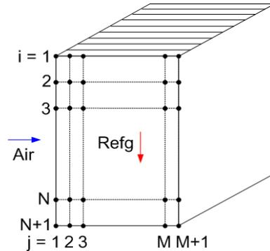
**Figure 2:** Discretization of heat exchanger
