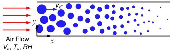
**Figure 1:** Schematic of the mist evaporative precooling method
