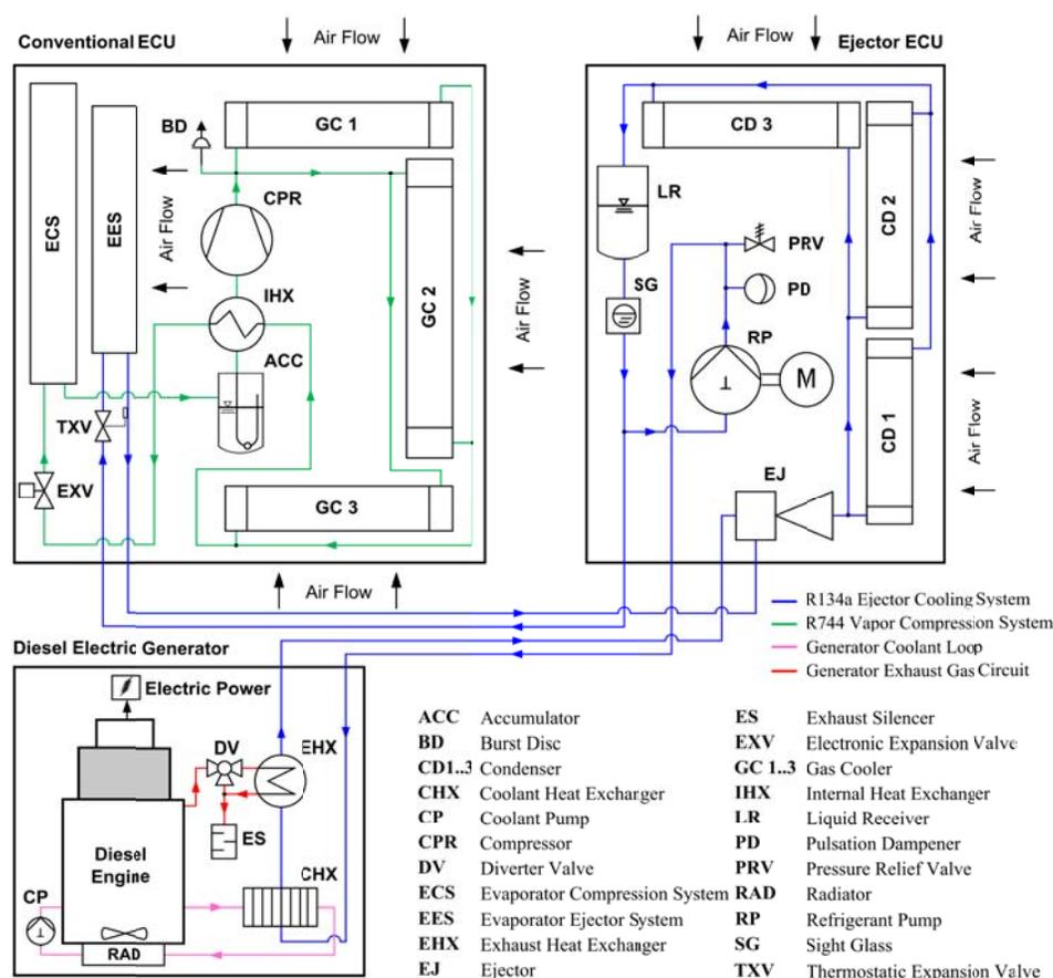
**Figure 2:** Schematic of the trailer-mounted integrated waste heat recovery ejector system
