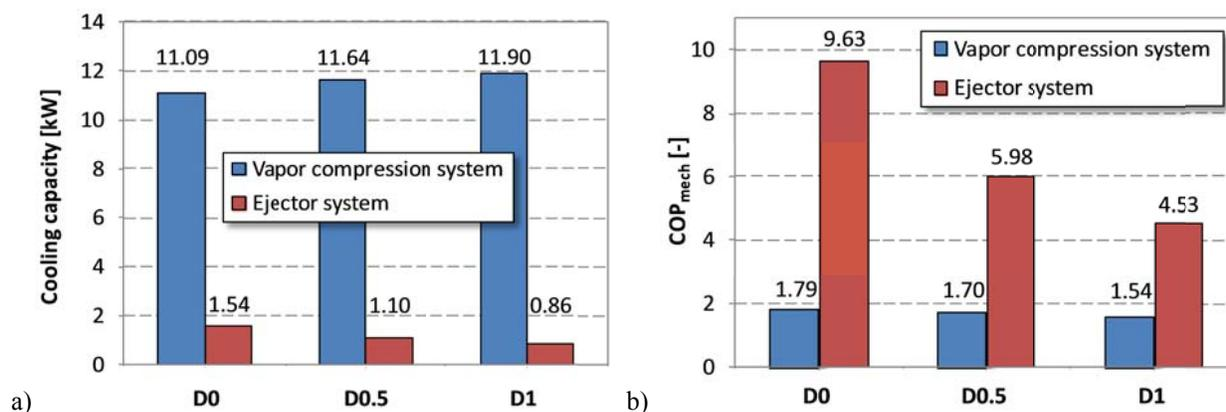
**Figure 8:** Comparison of a) cooling capacity and b) COP<sub>mech</sub> between the conventional and vapor jet ejector system at various ambient temperature conditions
