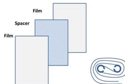
**Figure 5:** Polymer foils heat exchanger
