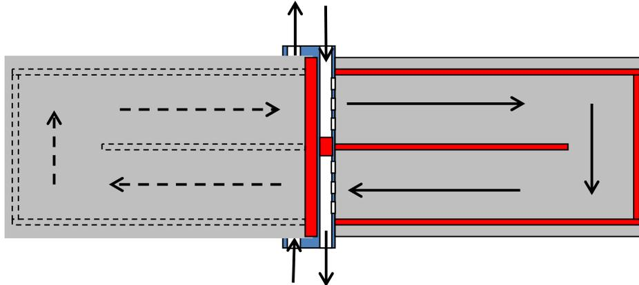
**Figure 6:** Basic design of a spiral HEX using polymer films
