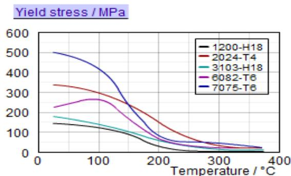
**Figure 3:** Reduction of yield stress of aluminum with temperature /ALU/
