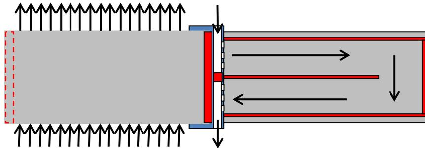
**Figure 7:** Basic design of a spiral HEX for gas / liquid applications using polymer films
