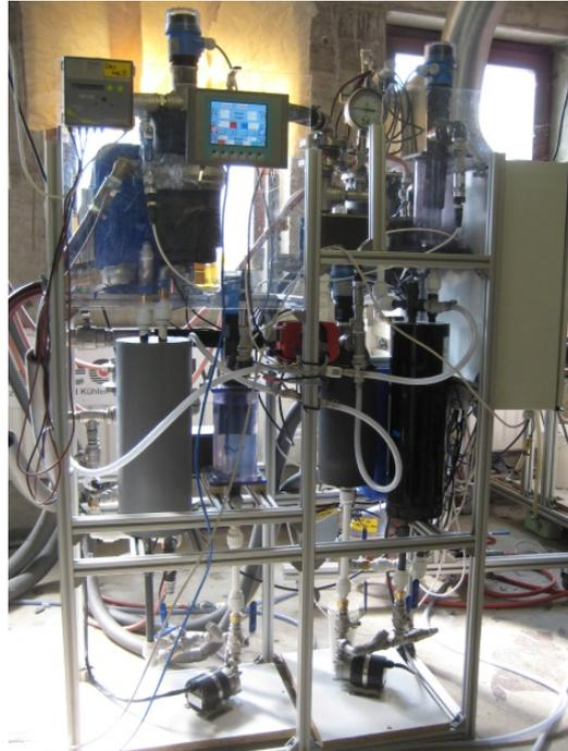
Figure 8: Resorption plant with two polymer HEX as solution heat exchanger
