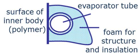
**Figure 2:** Evaporator tube and inner liner of a refrigerator with integrated evaporator
