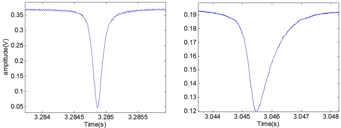
Figure 2.5 (a) A symmetric resonance captured by the oscilloscope. (b) Shows an asymmetric resonance.
