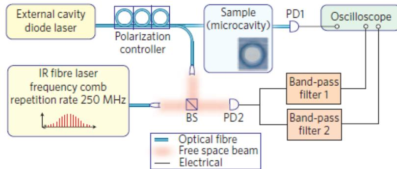
Figure 2.2 Experimental setup for measuring dispersion, reproduced from [3]
