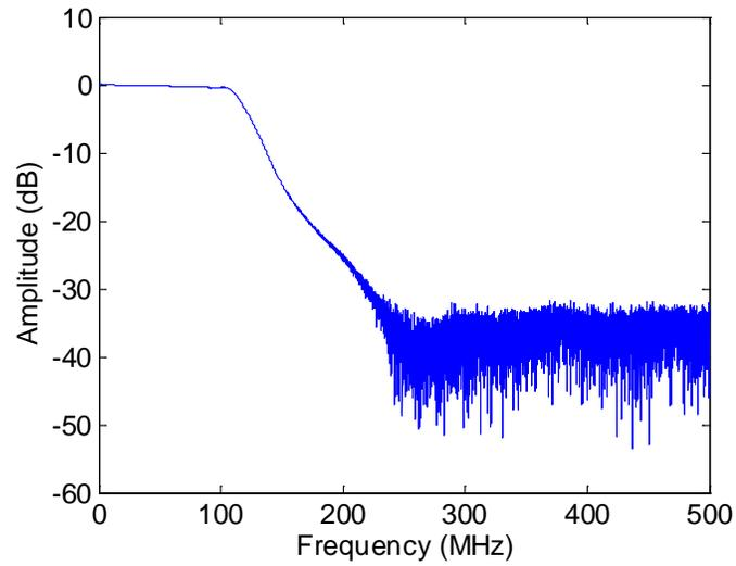
Figure 2.9 Frequency response of the low pass filter.
