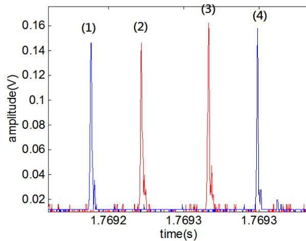
Figure 2.12 Example of one set of frequency marker. No error if peak (1) to (4) is in the right order.
