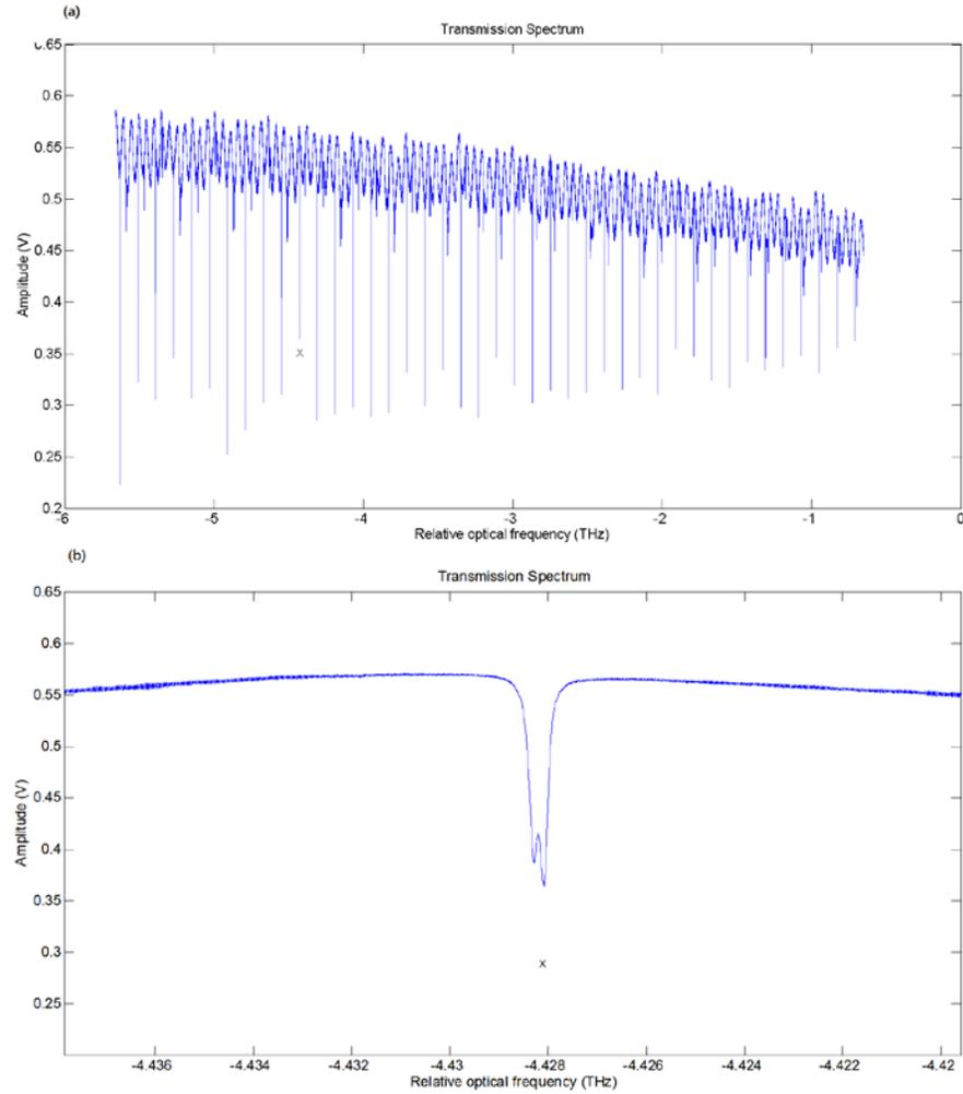
Figure 3.2 Transmission spectrum of the device with  $430\text{nm} \times 2\mu\text{m}$  dimension. (a) The transmission spectrum of the device. The x axis is the relative frequency obtained by frequency marker. The real frequency is unknown since the reference laser wasn't included. (b) Zoom in view of the peak mark as 'x' in (a). The peak has double peak feature, so we exclude that from our FSR fitting.
