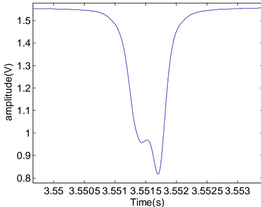
Figure 2.10 Double peak resonance is sometimes found in the transmission spectrum. The location of peak can't be determined.
