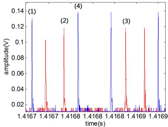
Figure 2.13 First 30MHz peak has smaller amplitude and is not recognized as a marker. The index difference of (4)-(3) will be negative and we can tell one of the peak is missing.
