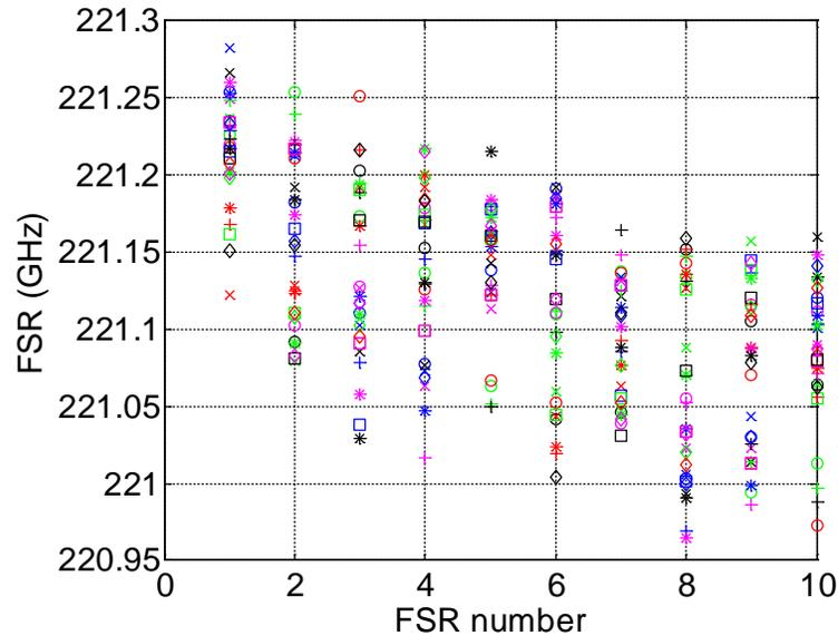
Figure 3.10 FSR deviations for the resonances from 1540nm to 1560nm. The maximum deviation of the FSR is around 200MHz.
