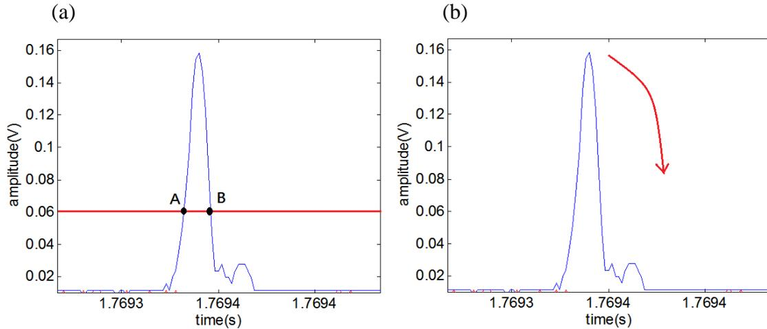
Figure 2.11 (a) A minimum threshold is set to distinguish frequency marker from noise background. Point A is defined to be start of a frequency marker and B is end of frequency marker. (b) A small jump is introduced to avoid the transient response of the band-pass filter is captured as well.
