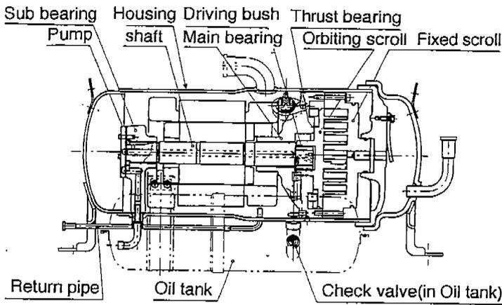
Fig.1 Structure of horizontal scroll compressor
