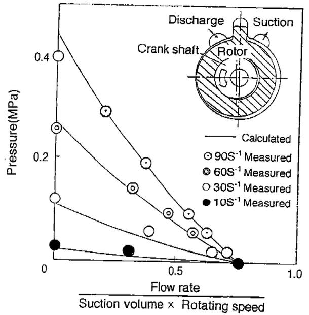
Fig.2 Structure and characteristics of displacement type oil supply pump
