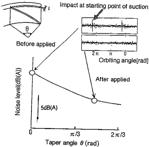
Fig.7 Reduction of impact noise by smoothing contact force between walls
