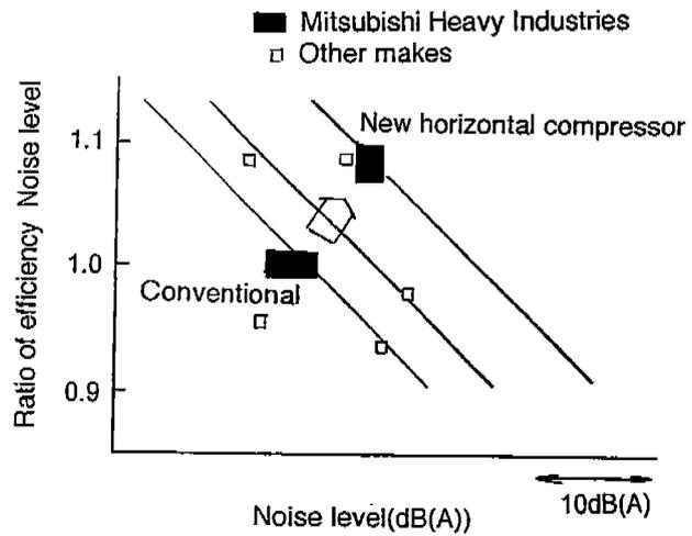
Fig.8 Realization of high efficiency and low noise in new scroll compressor
