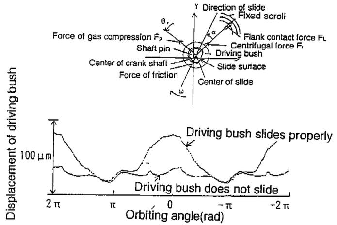
Fig.6 Behavior of driving bush in sliding type variable crank radius mechanism
