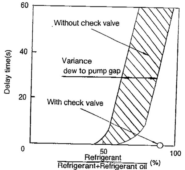
Fig.4 Delay time of oil supply at compressor starting
