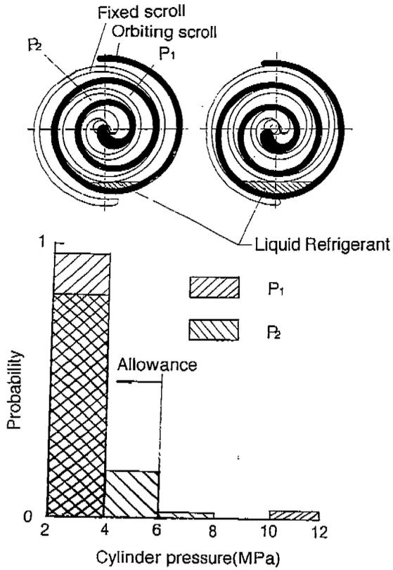
Fig.5 Distribution of probability of cylinder pressure
