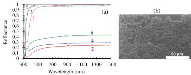
FIG. 5. (a) Reflectance spectra (front illumination) of a metamaterial consisting of three pairs of Ag/MgF<sub>2</sub> layers, deposited on a flat substrate (trace 1), and on glass microspheres (trace 2). Traces 3 and 4—same for a metamaterial consisting of six pairs of Ag/MgF<sub>2</sub> layers. Traces 5 and 6—same for a silver film. (b) Scanning electron microscope (SEM) image of a lamellar metamaterial deposited onto glass microspheres.
