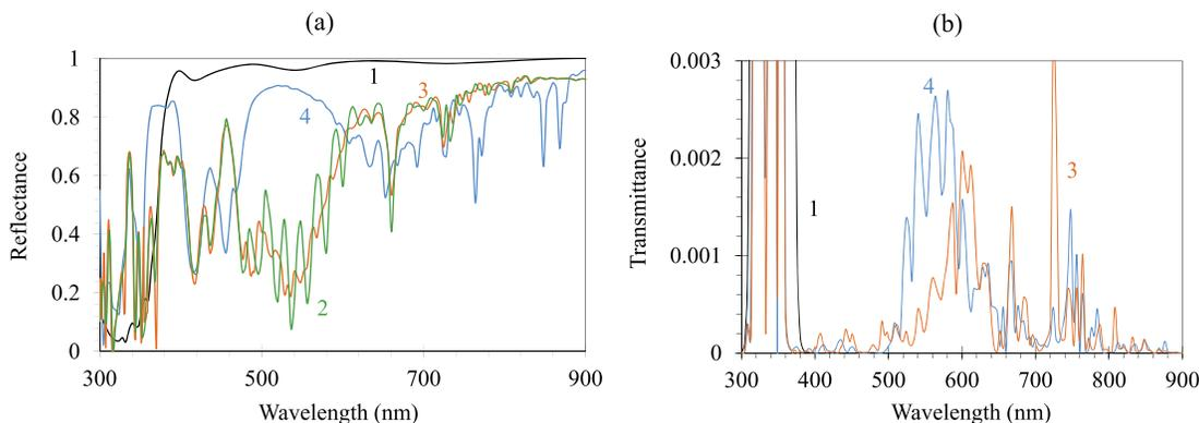
FIG. 4. (a) Calculated reflectance spectra of a lamellar Ag/MgF<sub>2</sub> metamaterial with no nanoparticles (trace 1), with 200 nm TiO<sub>2</sub> nanoparticles on the top (trace 2), with 200 nm nanoparticles on the top and 100 nm nanoparticles at the bottom (trace 3), and with 100 nm nanoparticles on the top and 200 nm nanoparticles at the bottom (trace 4). (b) Calculated transmission spectra of the samples 1, 3, and 4 from (a).
