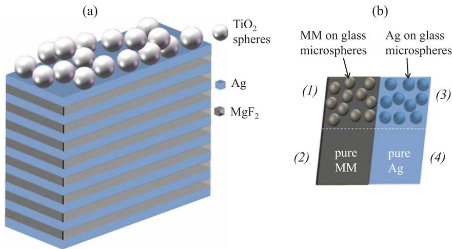
FIG. 1. (a) Schematic of a lamellar Ag/MgF<sub>2</sub> hyperbolic metamaterial used in the experiments (Ag ~25 nm, MgF<sub>2</sub> ~35 nm), with 330 nm TiO<sub>2</sub> nanoparticles deposited on the top. (b) Schematic of a microsphere-based sample containing four principle areas: (1) multilayered metamaterial on top of microspheres, (2) multilayered metamaterial on top of glass, (3) silver on top of microspheres, and (4) silver on top of glass.
