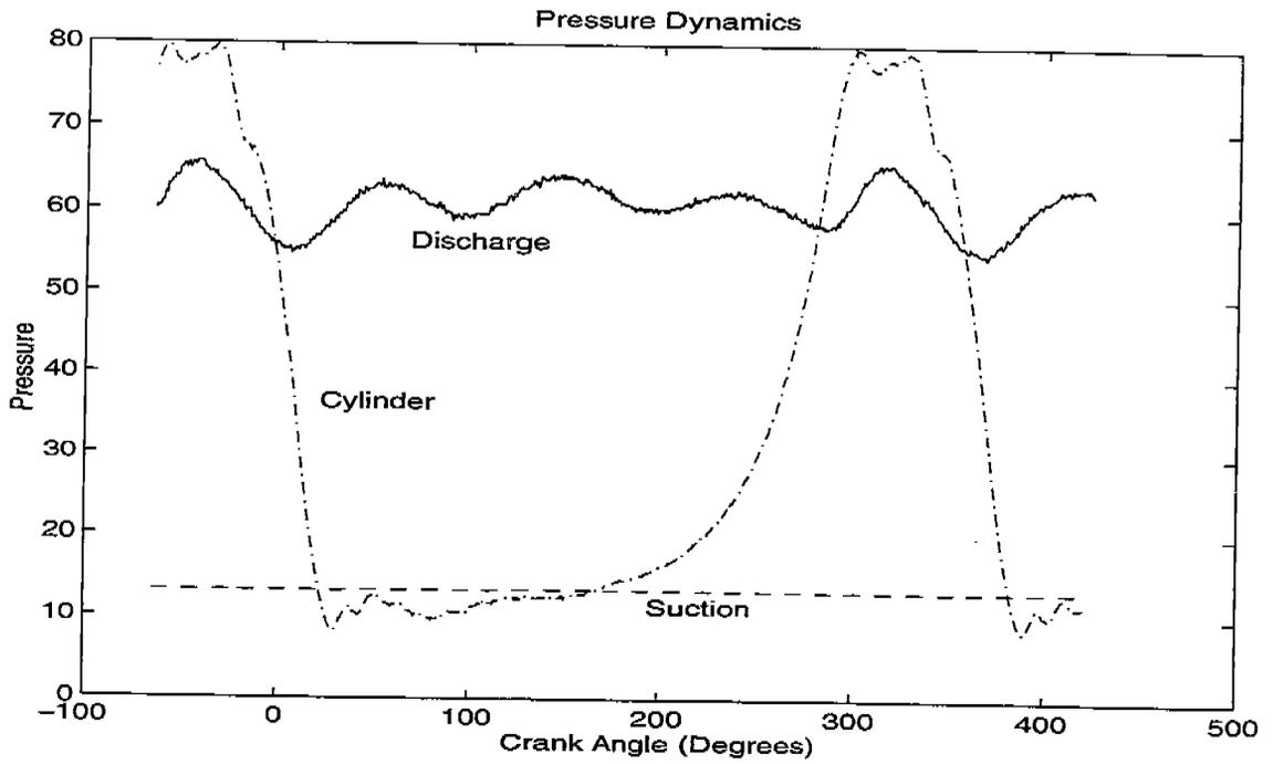
Figure 5: Compressor Pressure Data
