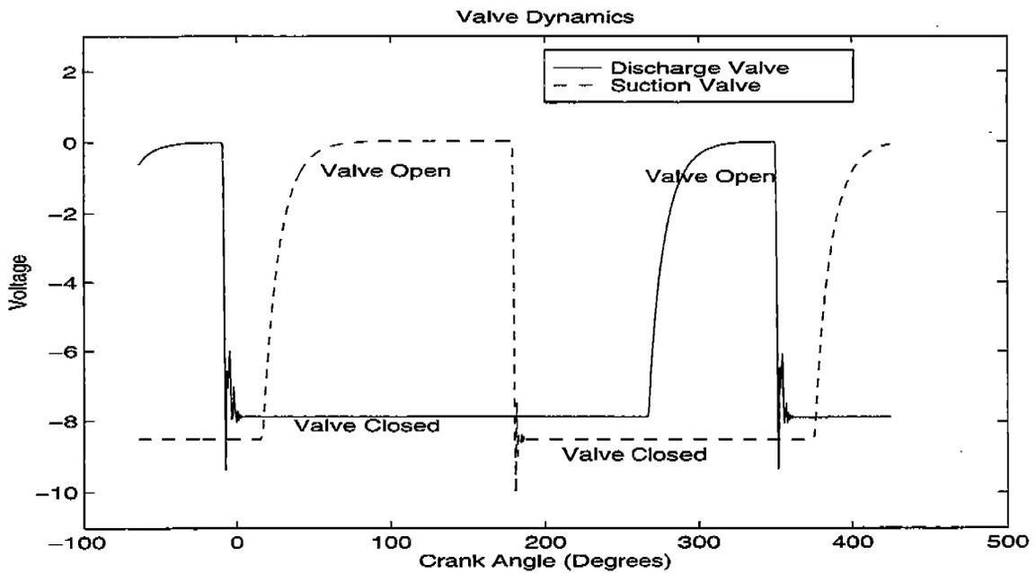
Figure 3: Measurement of Valve Lift
