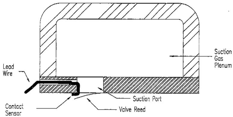
Figure 1: Contact Sensor Setup.
