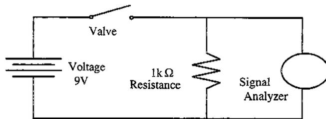
Figure 2: Contact Sensor Electrical Circuit Setup
