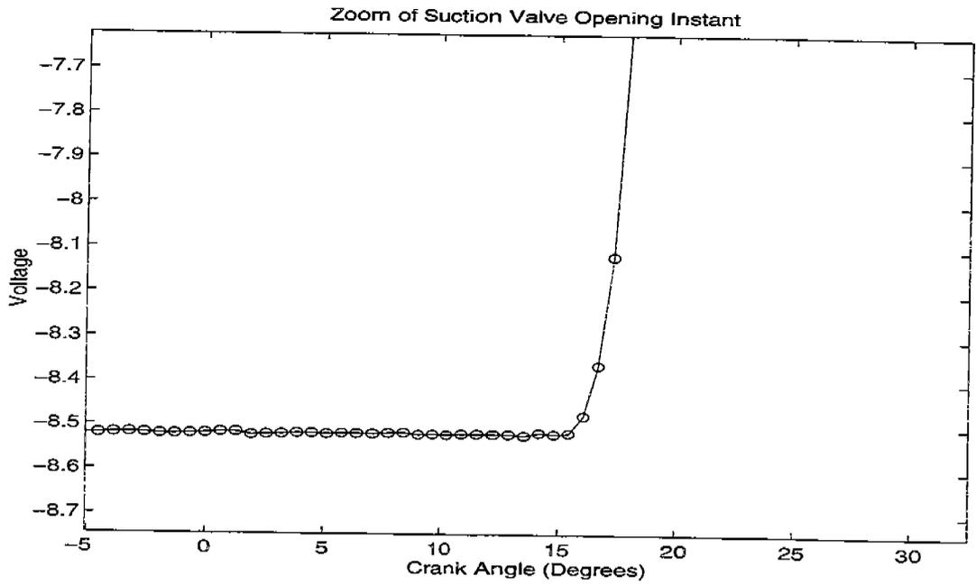
Figure 4: Zoom of Suction Valve Data at Instant of Valve Opening
