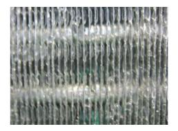
Figure 13: The surface state of cross stair slit fin (on wet surface condition)
