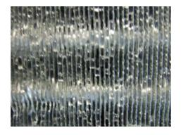
Figure 12: The surface state of ring fin (on wet surface condition)
