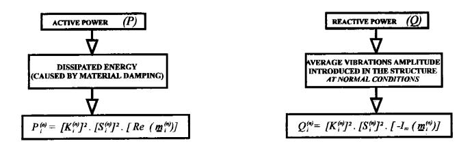
i = 1,2,3 (direction) (n).=. n° structure point where is supposed exisisting an pump anchorage point Ki = stiffness value of the connecting spring
