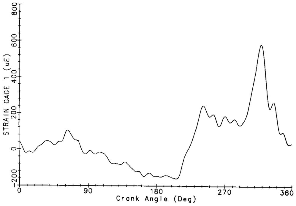
**Figure 5 Strain Versus Crankangle**
