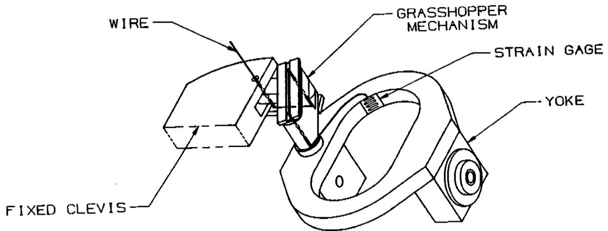
**Figure 4 "Grasshopper" Mechanism Attached to Scotch Yoke**
