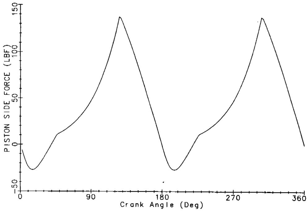
**Figure 2 Piston Side Force Versus Crankangle**
