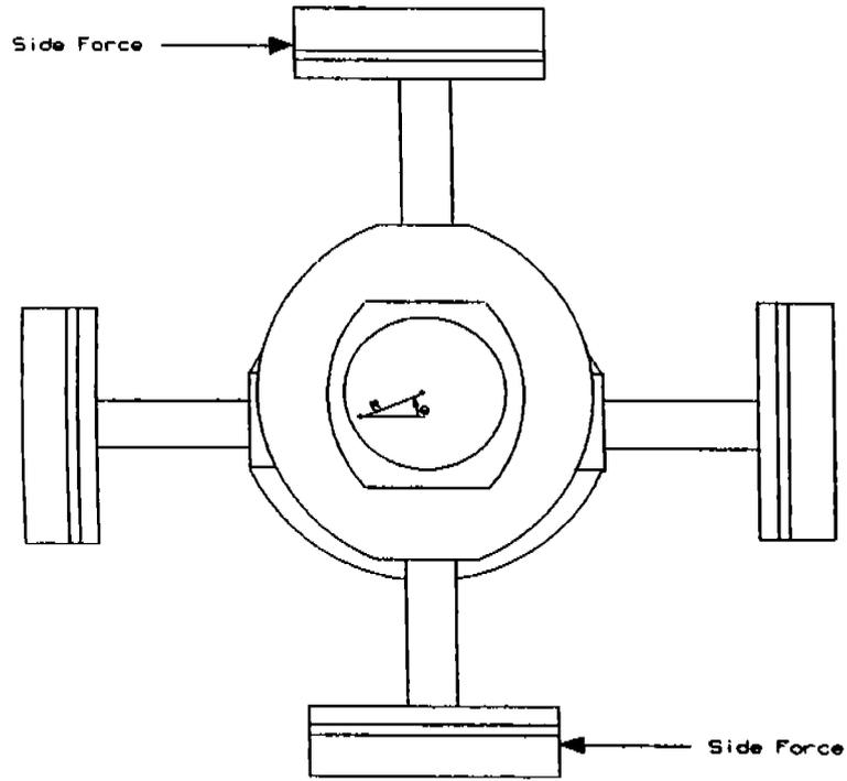
**Figure 1 Schematic of Scotch Yoke Mechanism With Piston Side Force**
