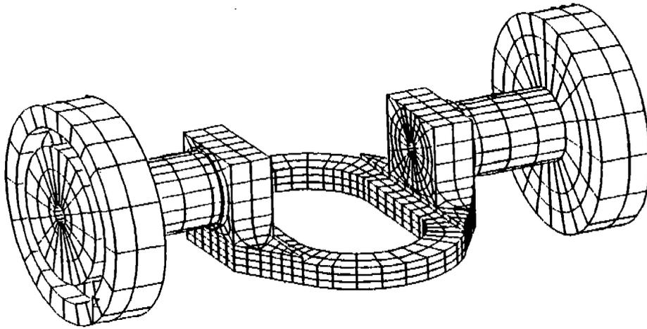
**Figure 3 Finite Element Model of Scotch Yoke**
