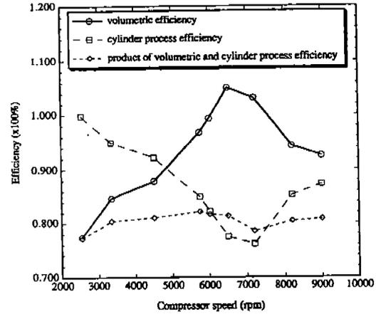
Figure 6 Comparison among volumetric efficiency, cylinder process efficiency, and their product ( $p_1=63.5$  psia,  $T_1=45.5$  F,  $p_2=242$  psia)
