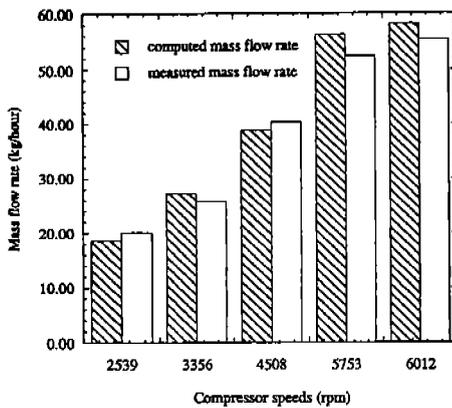
Figure 7 Mass flow rate comparison ( $p_1=63.5$  psia,  $T_1=45.5$  F,  $p_2=242$  psia)
