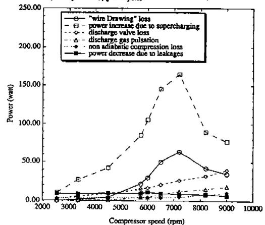
Figure 4 Power variation under different speeds ( $p_s=63.5$  psia,  $T_s=45.5$  F,  $p_d=242$  psia)
