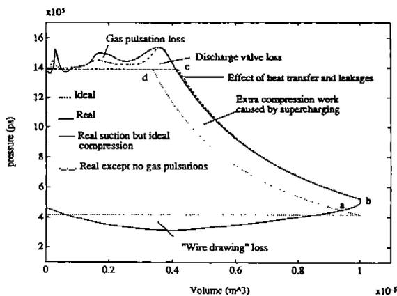
Figure 3 Energy losses on PV diagram ( $\Omega=6550$  rpm,  $p_s=418511.76$  pa,  $T_s=42.9$  F,  $p_d=1388604.1$  pa)
