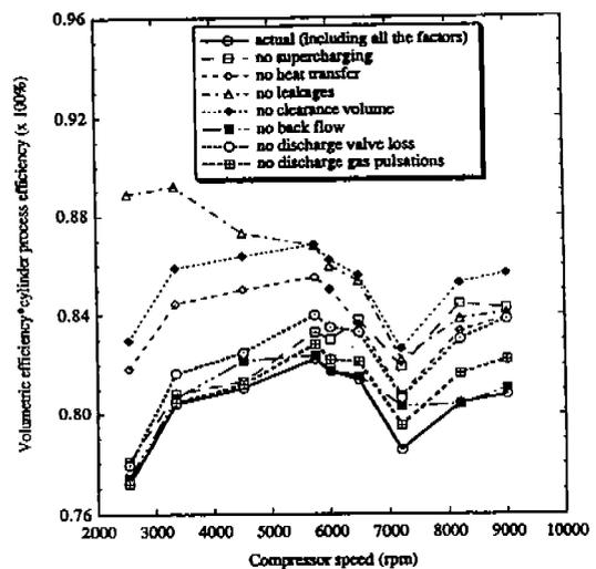
Figure 10 Product of volumetric efficiency and cylinder process efficiency under different situations ( $p_1=63.5$  psia,  $T_1=45.5$  F,  $p_2=242$  psia)
