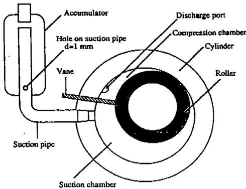
Figure 1 A rolling piston rotary compressor mechanism
