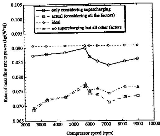
Figure 9 Ratio of mass flow rate to the corresponding power required for the cylinder processes ( $p_1=63.5$  psia,  $T_1=45.5$  F,  $p_2=242$  psia)
