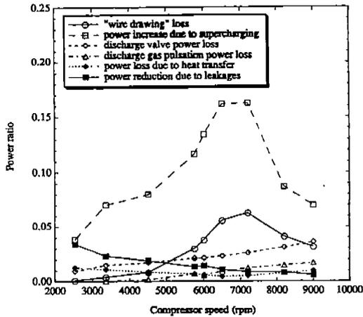
Figure 5 Ratios of the power variations to the total power needed for the cylinder processes ( $p_1=63.5$  psia,  $T_1=45.5$  F,  $p_2=242$  psia)
