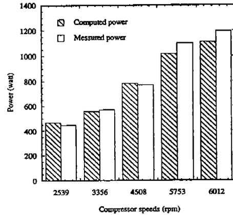
Figure 8 Total power consumption of the test compressor
