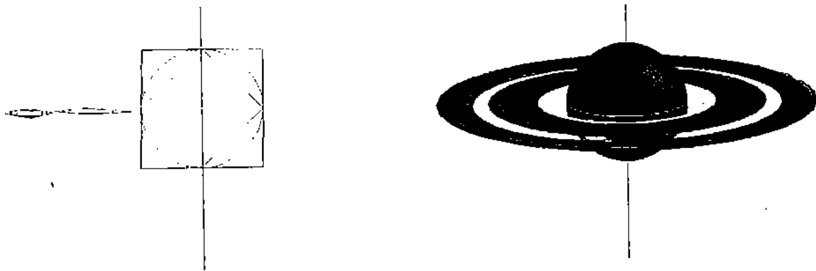
Figure 6.2: A C^2 A-spline and Revolution Surface
