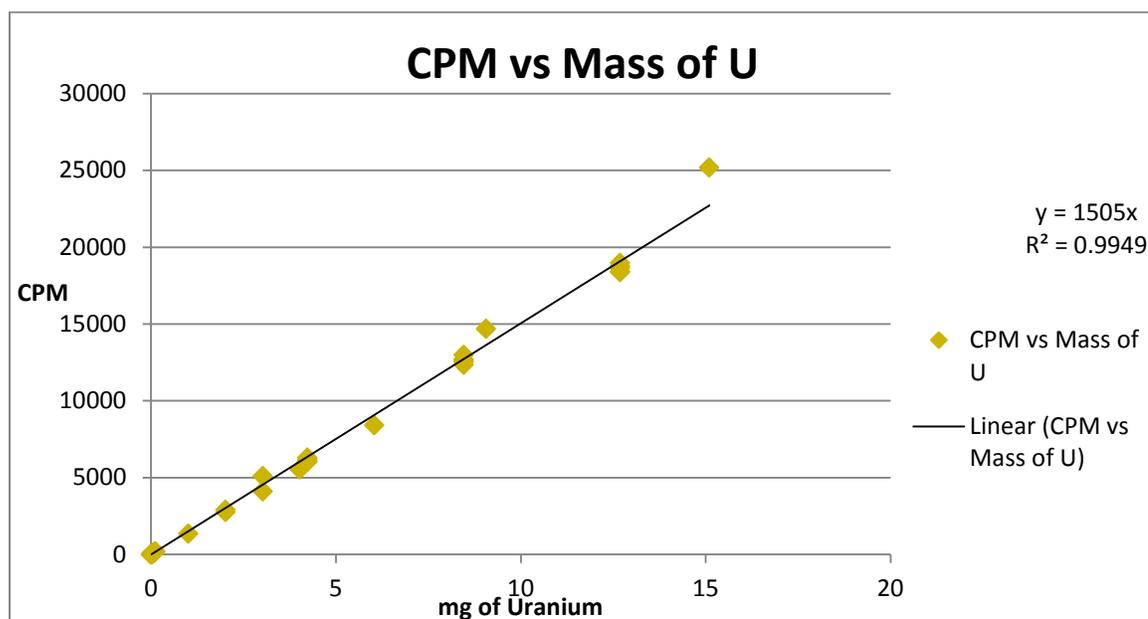
Figure 14 LSC CPM versus Mass of Uranium
