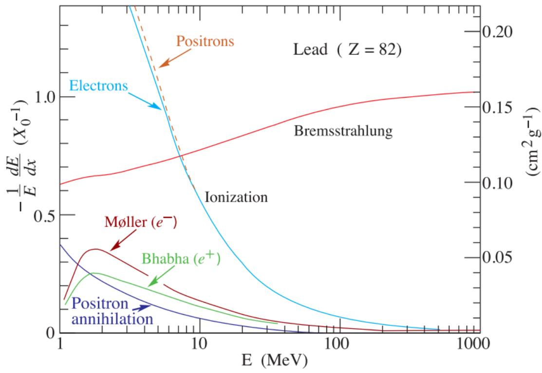
Figure 3 Fractional Energy Loss per Radiation Length in Lead (<http://pdg.lbl.gov/>)
