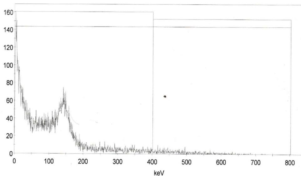
Figure 13 Perkin Elmer TriCarb 2800 Uranyl Nitrate Spectrum
