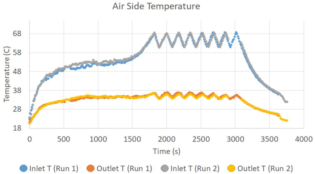
Figure 5: Air Side Inlet and Outlet Temperatures of Heat Exchanger
