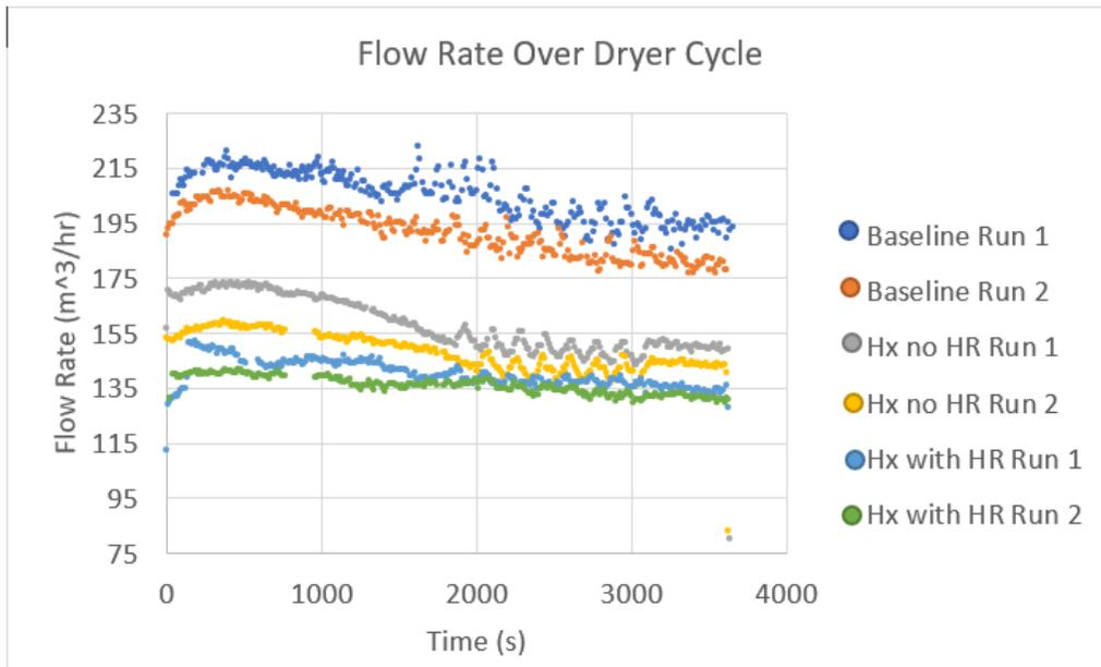
Figure 4: Flow rates of moist air stream in dryer duct
