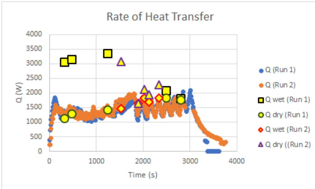
Figure 8: Model Heat Transfer Rate Compared with Experimental Data Heat Transfer Rates
