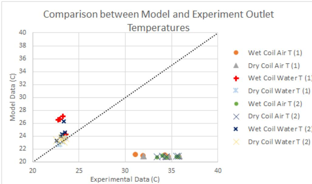
Figure 7: Comparison Between Specific Experimental Values and Corresponding Model Outputs
