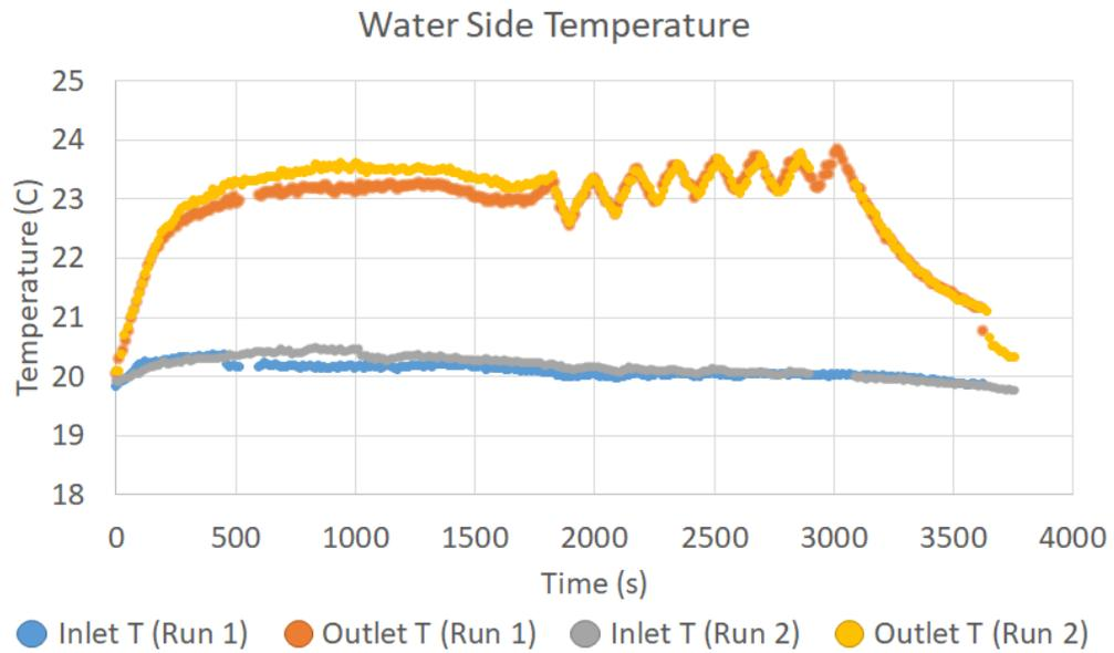
Figure 6: Water Side Inlet and Outlet Temperatures of Heat Exchanger
