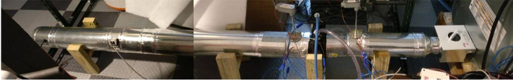
Figure 2: Physical Layout of Dryer Duct
