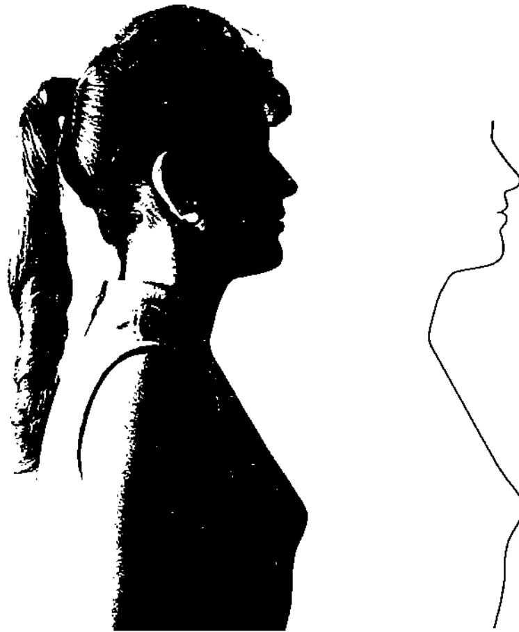
Figure 7: Photograph (left) of a girl and an approximation (right) to the profile. The approximation is a cubic spline with 16 polynomial pieces computed in 1963 at the General Motors Research Laboratories.
