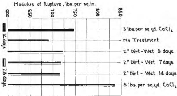
Fig. 2. Transverse strength at 14 and 28 days.
