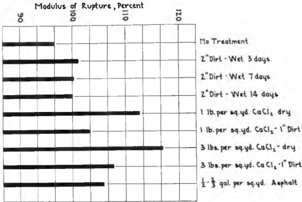
Fig. 1. Transverse strength of specimens at 28 days.
