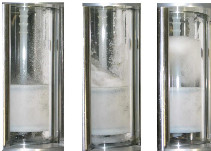
Figure 3: Mass flow through a clear high pressure side receiver under steady state operation and constant boundary conditions. Total system charge increases from left to right: 400g, 700g and 1200g.
