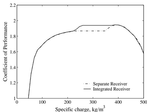
Figure 6: Simulation results of the Coefficient of Performance indicate an optimum refrigerant charge and dependence on receiver position
