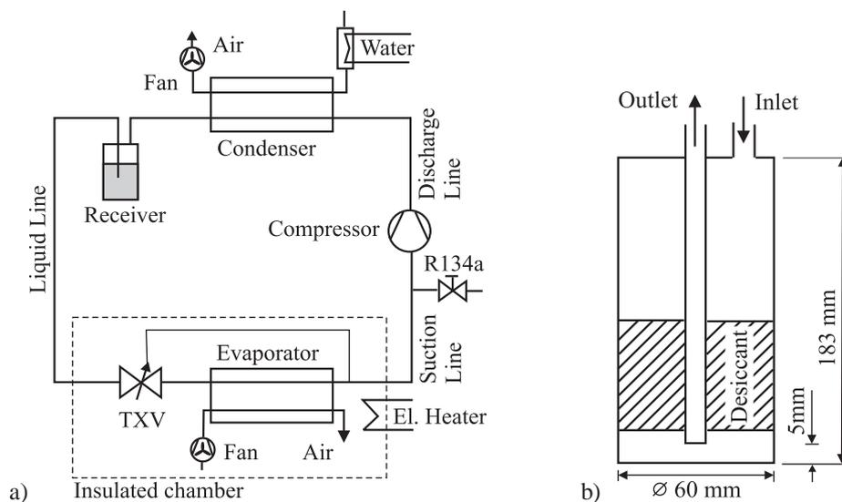
Figure 1: a) schematic of the experimental setup, b) high pressure side receiver
