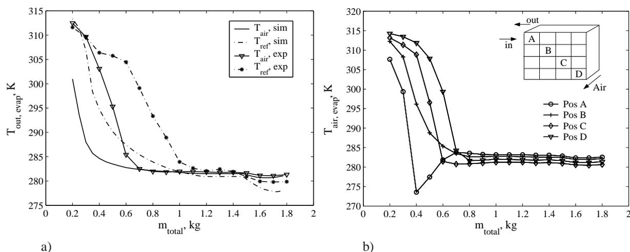
Figure 5: a) air and refrigerant outlet temperatures at the evaporator vs. total system charge. b) measured evaporator air outlet temperatures at different sensor positions vs. total system charge
