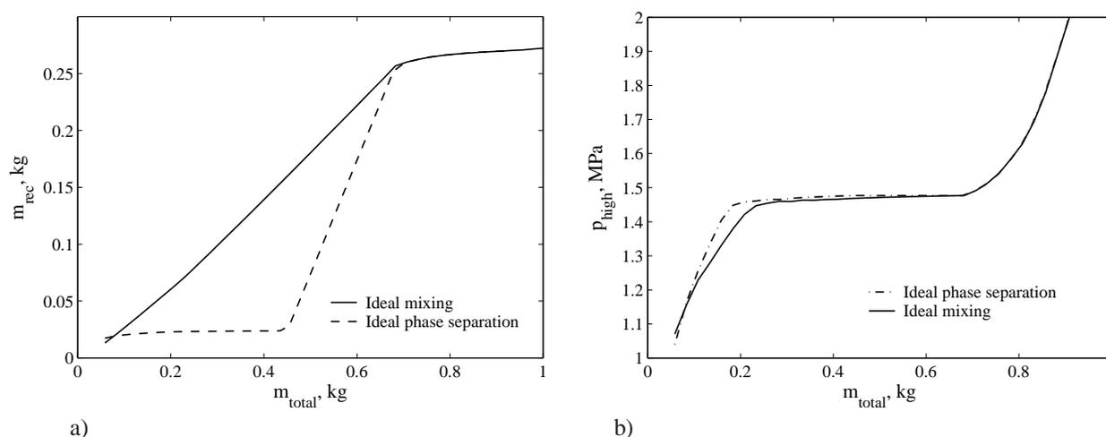
Figure 2: Mass accumulation (a) and discharge pressure (b) vs. the total charge in a system simulated with different receiver models.
