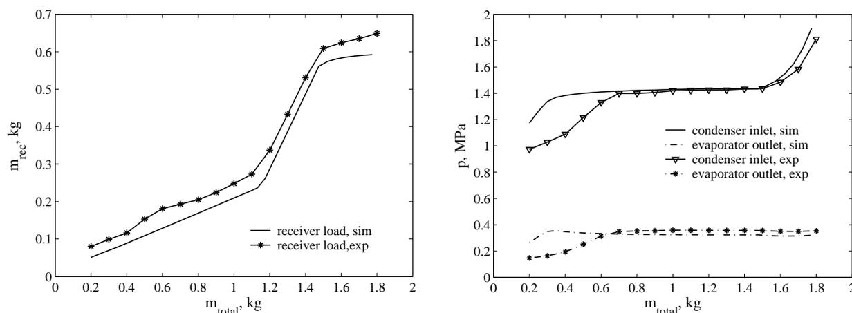
Figure 4: Refrigerant mass in the receiver and system pressures vs. total system charge, simulation and experiment
