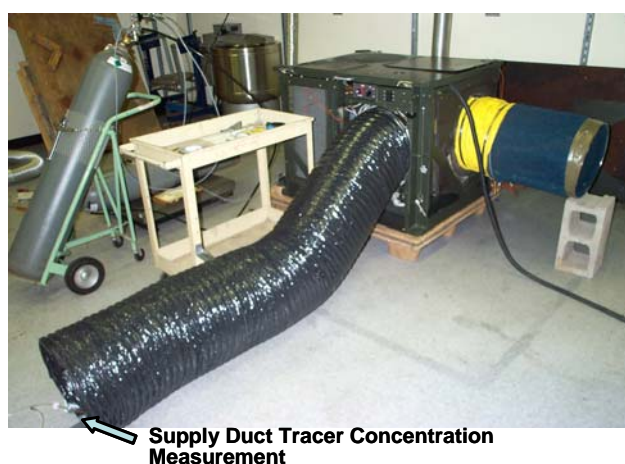
Figure 6: LECU in Tracer Gas Test
