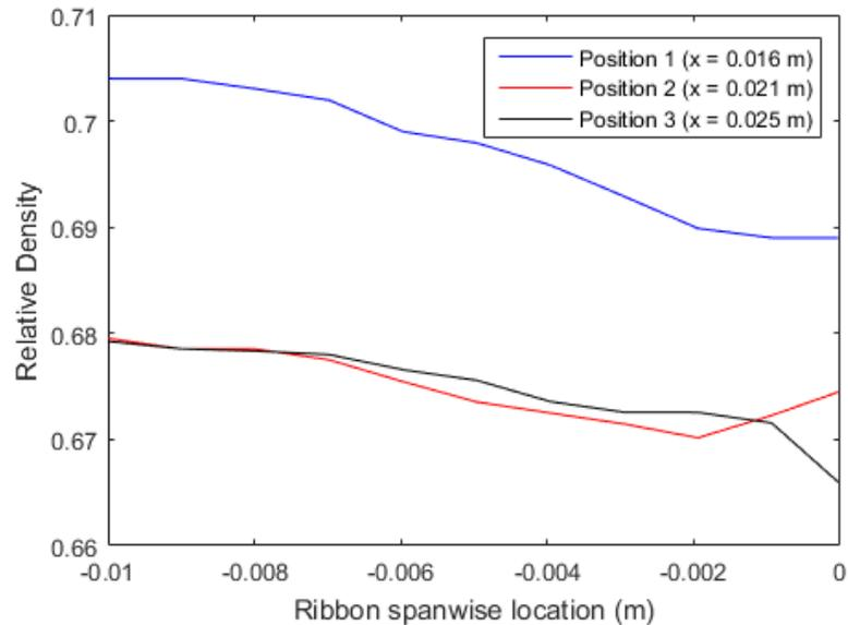
Figure 4.5. Relative density along the ribbon spanwise direction based on distance from the cheekplate (with zero closest to the cheekplate) for different positions shown in Figure 4.4.
