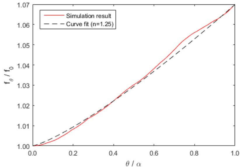
Figure 5.6. The mass correction factor normalized by the mass correction factor at  $\theta = 0$  plotted as a function of angular position normalized by the nip angle as measured from FEM simulations for powder-cheekplate friction coefficient of (a) 0.15 and (b) 0.35. The curve fits proposed in Equation (12) for different exponent  $n$  are shown as dashed lines.
