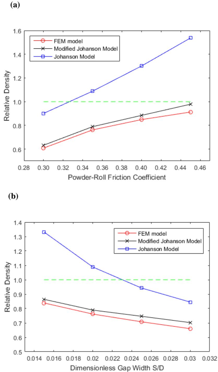
Figure 5.5. Maximum relative densities as functions of (a) powder-roll friction coefficient and (b) dimensionless gap width  $S/D$ . The inlet stress, minimum gap width, roll diameter, and powder-roll friction coefficient are, respectively, (a) 200 kPa, 4 mm, 200 mm, N/A and (b) 200 kPa, N/A, 200mm, 0.35. The remainder of the material properties are given in Tables 3.2 and 3.3.
