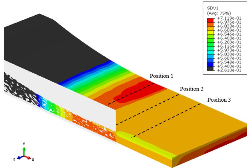
Figure 4.4. Relative density distributions for the example simulation with the release region extending downstream of the side plates. The inlet stress, minimum gap width, roll diameter, roll width, powder-roll friction coefficient, and powder-cheekplate friction coefficient for this special case are, respectively, 200 kPa, 2 mm, 100 mm, 20mm, 0.35, and 0.35. The remainder of the material properties are given in Tables 3.4 and 3.5.
