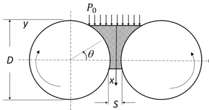
Figure 1.1. Roll compaction.
