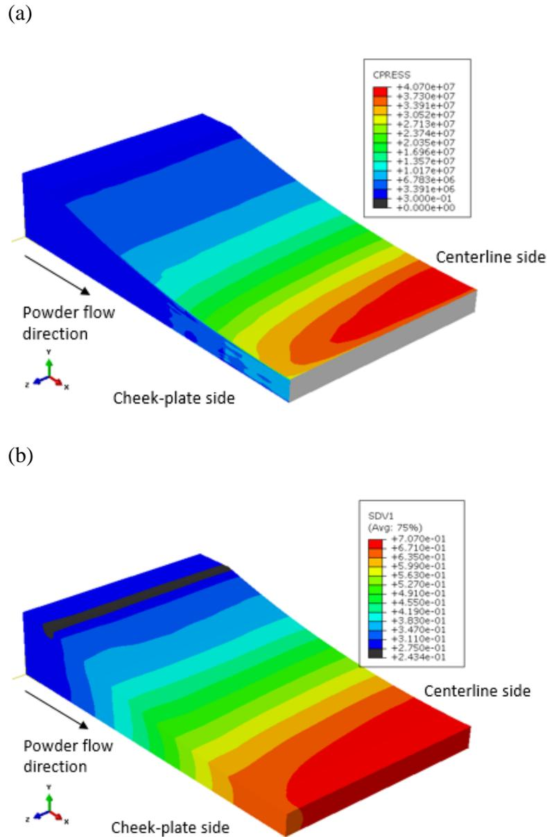
Figure 4.2. (a) Roll normal stress (Pa) and (b) Relative density distributions for the example simulation. The inlet stress, minimum gap width, roll diameter, roll width, powder-roll friction coefficient and powder-cheekplate friction coefficient for this special case are, respectively, 200 kPa, 2 mm, 100 mm, 20mm, 0.35 and 0.35. The remainder of the material properties are given in Tables 3.4 and 3.5.
