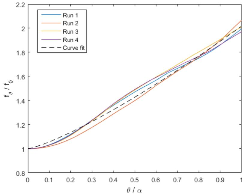
Figure 5.3. The mass correction factor normalized by the mass correction factor at  $\theta=0$  plotted as a function of angular position normalized by the nip angle as measured from FEM simulations (Table 5.1). The curve fit proposed in Equation (5.16) is shown as a dashed line.
