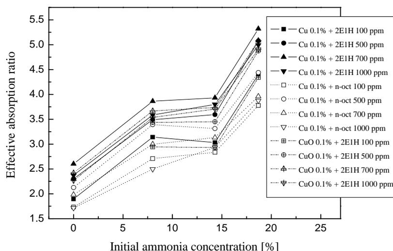
Figure 6 : The Effective Absorption Ratio for the Binary Nanofluids with Surfactants
