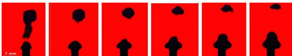
Figure 5 : The bubble absorption behavior in the copper 0.1% binary nanofluid with 2-ethyl-1-hexanol 700ppm
