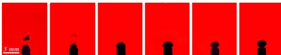
Figure 4 : The bubble absorption behavior in the copper 0.1% binary nanofluid
