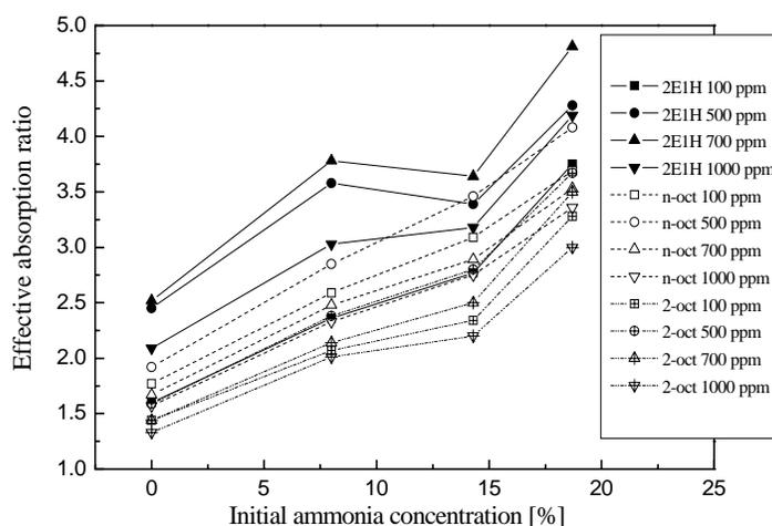
Figure 2 : The Effective Absorption Ratio for the addition of Surfactants
