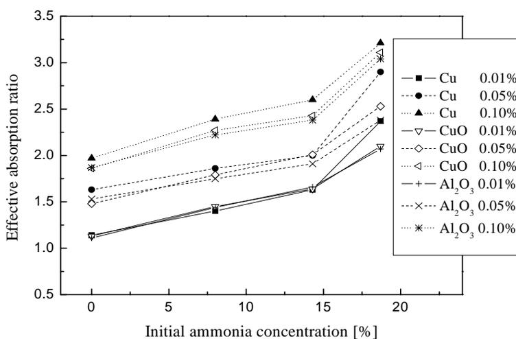
Figure 3 : The Effective Absorption Ratio for the addition of Nanoparticles
