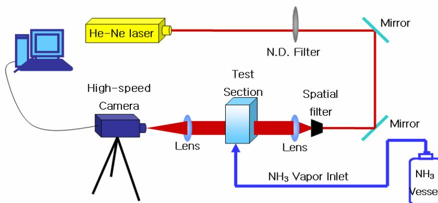
Figure 1 : Schematic Diagram of Visualization Apparatus
