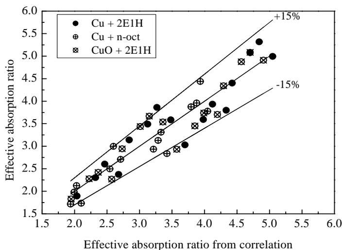
Figure 7 : The experimental correlation of the effective absorption ratio for the binary nanofluids with surfactants
