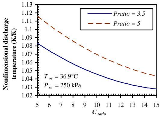
Figure 7: Curve fits of nondimensional compressor discharge temperature as a function of  $C_{ratio}$  for two  $P_{ratio}$  values.
