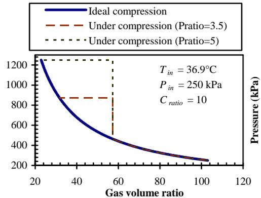
Figure 3: Pressure/volume ratio diagram showing under compression loss.
