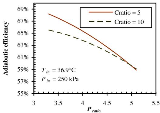
Figure 2: Experimental results for compressor adiabatic efficiency as a function of  $P_{ratio}$ .
