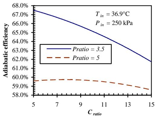
Figure 4: Compressor efficiency as a function of  $C_{ratio}$ .
