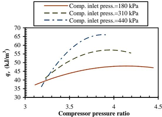
Figure 10: Cycle cooling capacity as a function of compressor pressure ratio for  $C_{ratio}=11$ .
