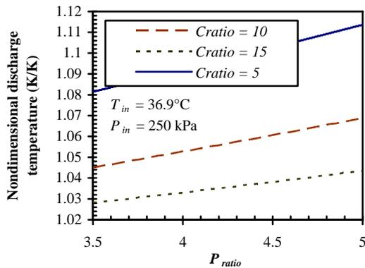
Figure 6: Nondimensional compressor discharge temperature as a function of  $P_{ratio}$  for three  $C_{ratio}$  values.
