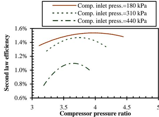
Figure 11: Cycle second law efficiency as a function of compressor pressure ratio for  $C_{ratio}=11$ .
