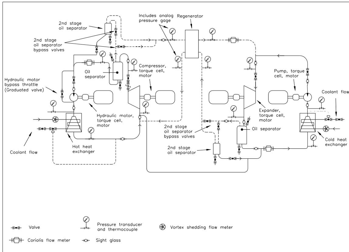
Figure 1: Schematic of the LFEC experimental system.
