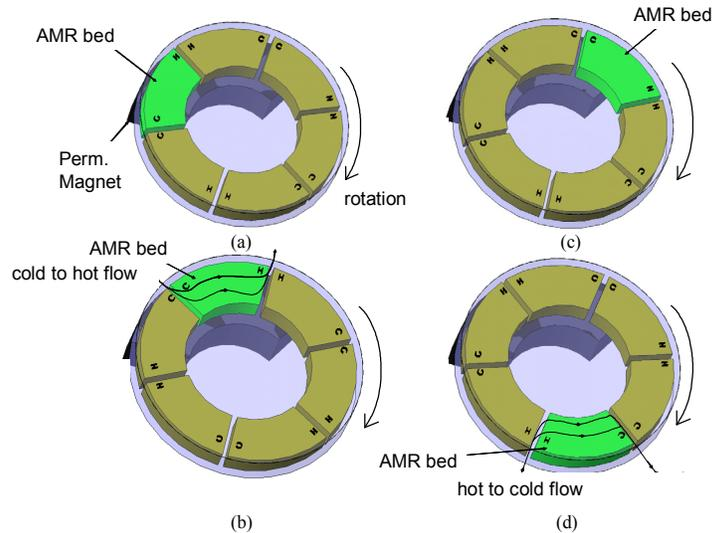
Figure 1: Conceptual drawing showing the processes that make up the rotary AMRR system: (a) magnetization, (b) cold-to-hot flow, (c) demagnetization, and (d) hot-to-cold flow.
